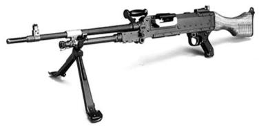
Maximum Effective Range Caliber System of Operation Overall Length Feed Device Weight (Loaded) 1,500 m 7.62-mm x 51 NATO Gas, automatic 1.26 m Belt 13.92 kg (with butt stock and bipod)
