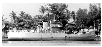
Complement Armament Maximum Speed (kts) Displacement (t) LOA/Beam/Draft m(f) 54 (4 officers). 2 x 12.7-mm MGs. 13. 1,034 full load. 54.9 x 11.3 x 3.8 (180 x 37 x 12).
