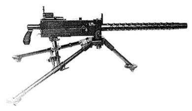
Maximum Effective Range Caliber System of Operation Feed 1000 m .30 caliber or 7.62-mm Automatic Belt
