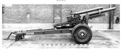
Crew 8 **Maximum Range** 11,270 m Rate of Fire 10 rds/min **Combat Weight** 2,030 kg Length 5.991 m Width 3.65 m Height 3.124 m Prime Mover 6 x 6
