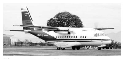
Transport Role Crew 3 25.8 m Wing Span Length 25.4 m Height 8.2 m Maximum T/O Weight 16,500 kg Maximum Speed 455 km/hr
