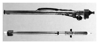
Guidance Maximum Range Combat Weight Length Passive IR homing Fm tracking logic seeker 4,500 m (inbound target) 5,200 m (outbound) 16.65 kg 1.7 m
