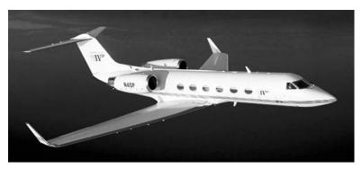
Role Transport, utility Crew/passengers 3/19 Wing Span 23.72 m Length 26.92 m Height 7.44 m Maximum T/O Weight 32.658 kg **Maximum Cruising Speed** 936 km/hr Maximum Range 6,667 km
