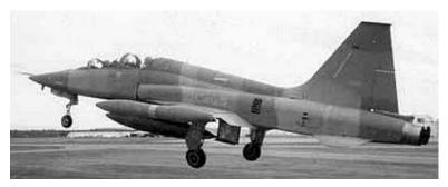
RoleLight Tactical Fighter (CF-5A)/Trainer (CF-5D)Armament2 x 20-mm guns; air-to-air missiles, surface-to-air missiles, and/or bombs.
