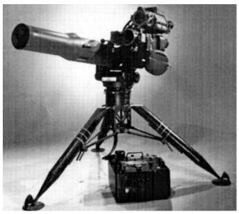
Diameter150 mmMaximum Range of Fire4 kmLength of Barrel1.17 mLaunch Weight19 kg
