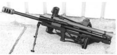
Maximum Effective Range Caliber System of Operation Overall Length Weight (Loaded) 1,800 m. 20-mm. bolt action, single shot. 1.33 m. 19.2 kg.
