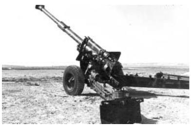
Crew 8 Maximum Range 27,150 m Rate of Fire 6 rds/min **Combat Weight** 7,700 kg Length 11.73 m Width 2.45 m 2.55 m Height Prime Mover 6 x 6
