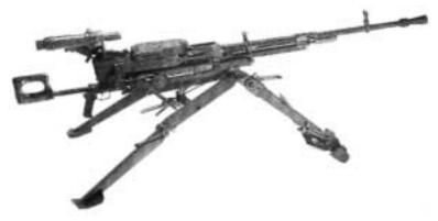
Maximum Effective Range Caliber System of Operation Overall Length Feed Weight 2,000 m 12.7 x 107-mm gas, automatic only 1.56 m 50-rd linked belt 57.9 kg
