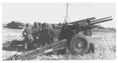
Crew 11 Maximum Range 14,600 m Rate of Fire 40 rds/h **Combat Weight** 5,760 kg 7.315 m Length Width 2.438 m Height 1.803 m Prime Mover 6 x 6
