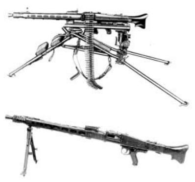
Maximum Effective Range Caliber System of Operation Overall Length Magazine Capacity Weight 800 m 7.62 x 54-mm Gas, automatic 47.2 in. 100, 200, or 250-rd metallic link belt 19.8 lbs
