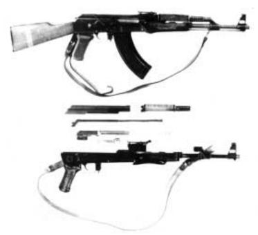
Maximum Effective Range Caliber System of Operation Overall Length Magazine Capacity Weight (Loaded) 400 m 7.62 x 39-mm Gas, selective-fire 34.25 in.
