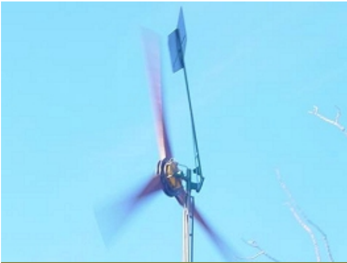
This photo shows a home-built 17-foot diameter 3.5 kW turbine with the tail in fully furling position. The machine is still making near maximum power, but it facing at an angle into the wind to reduce wind input. Photo by Dan Bartmann.
