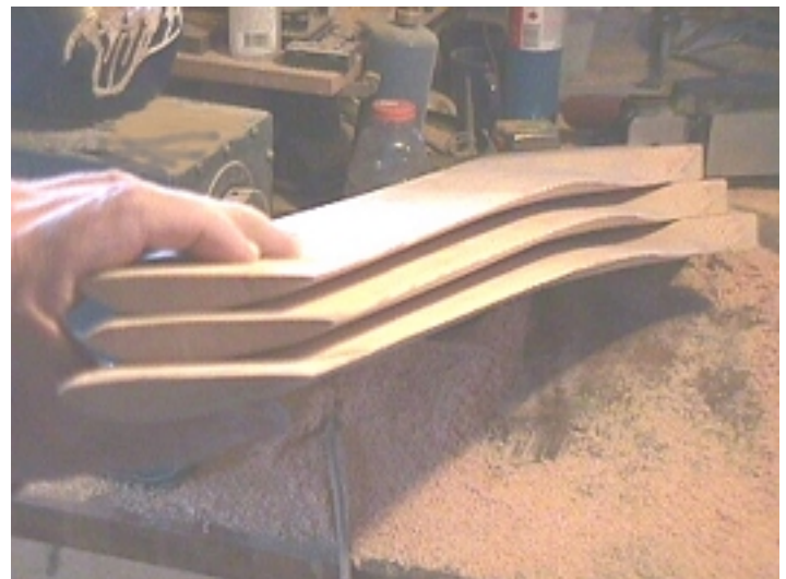
Freshly carved blades, showing the inherent twist that keeps the angle of attack correct from the tip to the root.
