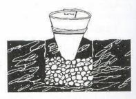
Incinerator: Rubbish should be burned. Make a fire in the latrine area using a large can as an incinerator. Bury unburned refuse in a pit.
