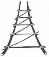
TRAVOIS: Choose two boughs with some spring to them and lash cross-pieces, as for the ladder. Add additional struts to provide closer support. Pull the load on its runners like a sled. (See also p. 245.)
