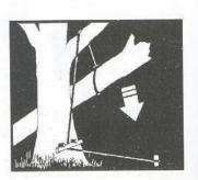
FIGURE 4 DEADFALL TRAP: Balance a horizontal bait bar at right-angles to an upright with a locking bar which supports a weight, positioned over bait, pivoted on sharpened tip of upright.
