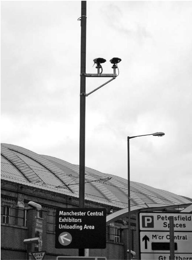
**Figure 10.6** ANPR cameras in central Manchester – installed in 2008
