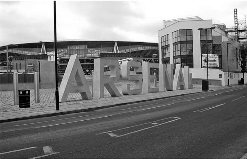
**Figure 10.11** The vehicle control barrier outside the Emirates Stadium, North London
