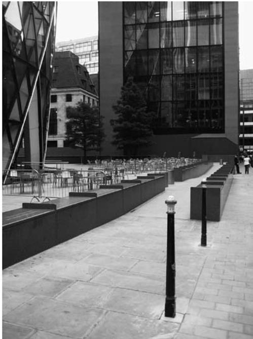
**Figure 10.10** The protective security features at the Gherkin in the City of London
