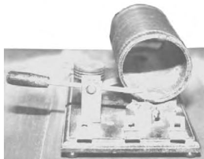
Left: A diagram of a crystal detector showing the round mounting base that holds a crystal, the catwhisker wire that makes physical contact with the crystal and transfers the vibrations to the main unit, and two leads for the headphones. Right: A crystal detector with a tuning coil, wound around a hollow cylinder, from the Bellingham Antique Radio Museum. [Classic Concepts, ©1997, used with permission.]
