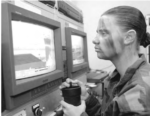
The display console and control panel for a Wide Angle Surveillance Thermal Imager in use at an air base in Korea. Airman 1st Class Olivia Latham scans the air traffic control tower for infiltrators during a scheduled rear area defense field training exercise. The background sky appears as a yellow color, while the large building on the left and control tower on the right show up as pink and lavender. [U.S. DoD 1999 news photo by Val Gempis, released.]
