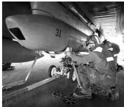
Left: Naval F-14 “Tomcat” aircraft were equipped with long-range AWG-9 radar systems which, when engaged, would apparently cause Iraqi MiGs to turn away. The Tomcat is shown here launching from an aircraft carrier in August 1999. Right: A Tactical Air Reconnaissance Pod System (TARPS) being removed from an F-14. [U.S. Navy news photos, released.]
