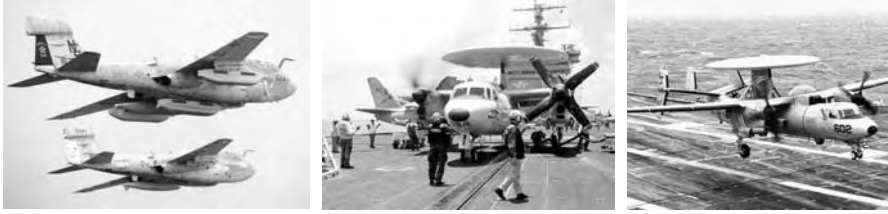
Left: The EA-6B Prowler was used for reconnaissance missions in Operation Desert Storm. Shown here are Prowlers patrolling the “No Fly” zone over southern Iraq in February 1998. The Prowlers provide ‘cover’ for accompanying planes and ships by jamming enemy radar systems, data links, and communications. Middle and Right: The radome , a protective radar cover, is clearly visible on this E2-C Hawkeye Airborne Early Warning aircraft. Hawkeyes provide long-range radar and communications support for aircraft carriers. [U.S. Navy photos by Chuck Radosta and Tedrick Fryman, III, Johnny Grasso, released.]
