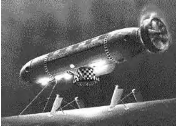
The DSRV Deep-Submergence Rescue Vehicle is designed to perform rescue operations on disabled, submerged submarines. They are designed to be easily transported and deployed by truck, aircraft, or marine vessel, or by an appropriately fitted submarine. This 15-meter Lockheed Missiles and Space, Co. vessel can dive up to approximately 1500 meters, conduct a search via sonar, and attach itself to the sub’s hatch in order to transfer up to 24 personnel to another location. It utilizes both search and navigation sonar systems. [U.S. Navy photo, released.]
