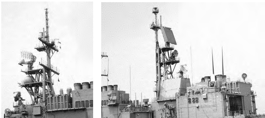
The U.S. Navy guided-missile destroyer USS Scott (DDG-995) is equipped (left) with an SPG-51 missile radar illuminator on top of the bridge, above which is a dome-shaped SPQ-9A surface gunfire-control radar, above which is an SPS-49(V)5 EW air search radar. Near the top of the mast is the SPG-55 surface-search antenna. To the aft end of the bridge is the SLQ-32(V)5 EW. The large screen (right) is the SPS-48E 3D search radar, below which is the SPG-60 gun/missile control. On the far right is a QE-82 antenna for WSC-3 UHF Satcomm. [U.S. DoD 1994 news photos by Don S. Montgomery, released.]
