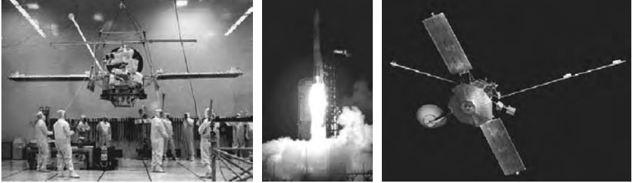
Left: Assembly of the Mariner 10 space probe. Middle: The launch in November 1973 on the Atlas Centaur launch rocket. Right: Artist's rendering of the Mariner 10 as it would have appeared during flight. The craft gathered data that indicated a thin atmosphere and magnetic field associated with the planet Mercury and earlier provided ultraviolet images of the Venutian atmosphere. [NASA 1973 news photos, released.]
