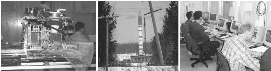
Left: Tests at Plesetsk necessitate the disassembly of the main avionics unit to fix a problem on the main processor board. Middle: The Astrid-2 Kosmos 3M rocket ready to launch in Plesetsk. Right: The Astrid-2 control center at the Swedish Space Agency headquarters at Solna, Sweden. [Swedish Space Agency 1998 and 1999 news photos, released.]
