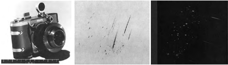
Left: The S-13 experimental Ultraviolet Astronomical Camera tested on the Gemini II space flight in 1966. The purpose of the experiment was to image the ultraviolet radiation from hot stars and to develop new ultraviolet photography techniques and devices. Middle and Right: Two frames of film from one of the early ultraviolet-sensing photography experiments that were carried out on the Gemini flight in August 1966. Black and white 70 mm film was used. [NASA/JSC news photo, released.]
