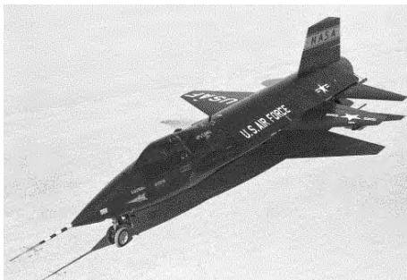
The X-15 was a rocket-powered, missile-shaped aircraft designed for high-altitude testing and the deployment of scientific sensing and data-collection instruments. Like the later Space Shuttle, the X-15 was launched from another craft at high altitude, in this case a B-52 aircraft (right). It would then glide in powerless flight and execute a glide landing. There is an X-15 rocket plane exhibited in the National Air and Space Museum in Washington, D. C. [NASA/ Dryden Flight Research Center 1960 and 1968 news photos, released.]
