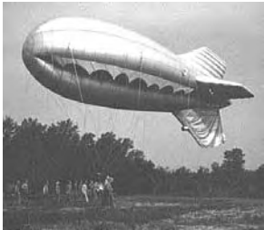
Left: U.S. Marine Corps with a barrage balloon on Parris Island, South Carolina in May 1942. The gas-filled barrage balloons and their cables were used as defensive obstacles to deter enemy reconnaissance and fighter aircraft. Right: Unfortunately, it's difficult to see them all in this small photo, but there appears to be a combination of at least a dozen airships and barrage balloons in this moving image of "D-Day" during World War II on the French beachhead in Normandy. [Library of Congress FSA/OWI photo by Alfred Palmer, public domain; U.S. Army 6 June 1944 historical archive photo by Steck, released.]
