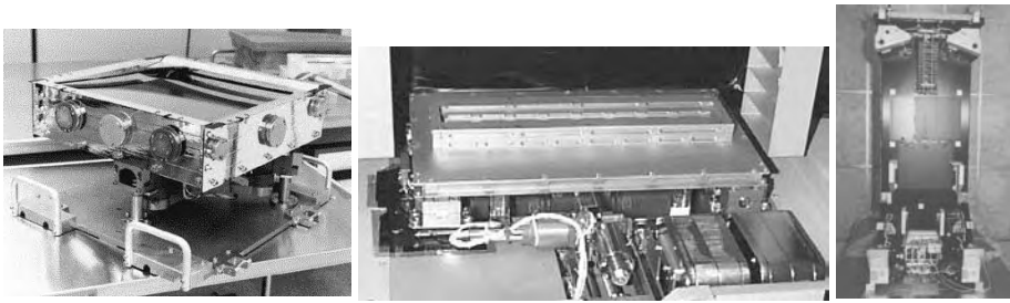
Left: One of four telescope mirror assemblies, assembled and tested in the 'clean room' at the Johns Hopkins University Homewood Campus. The light from the four mirrors is aligned and channeled into the spectrograph. Middle: One of the two detector assemblies, both of which serve as electronic 'retinas' to sense ultraviolet light and convert the energy into electrical signals that form the digital data that are communicated back to the Earth-based station. The sensors were constructed and tested at the University of California, Berkeley. Right: The FUSE spectrograph which contains the gratings (top) and detectors (bottom center) used to detect and analyze ultraviolet light. The spectrographic analyzer was assembled at the University of Colorado. [NASA 1998 news photos by Johns Hopkins University/APL; UC Berkeley; and University of Colorado, released.]
