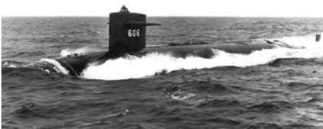
Left: The USS Timosa (SSN 606) is one of the Permit-class nuclear subs designed for quieter operation and greater stealth. These subs could also diver deeper than the older models. Right: The USS Thresher (SSN 593) was lost with all hands in 1963, possibly due to a defect in the piping system. Ironically, acoustics might have aided in detecting a possible defect, by more thorough application of ultrasonic testing to the joints and systems. [U.S. Navy news photo, public domain.]
