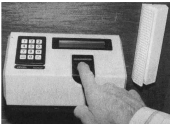
Figure 12-4. Fingerprint identification unit. A PIN is entered into the keypad and the index finger is placed on the center reader. The system then compares the fingerprint to one stored in a file to grant access.
