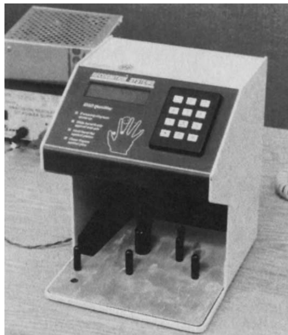
Figure 12-3. Hand geometry unit. The hand is placed on the platen and a small camera takes a picture. Specific measures are used to create a feature vector, which is compared to the stored user template.
