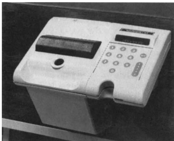
Figure 12-5. Retinal scan device. The user enters a PIN, then looks through the verifier and aligns a target. A scan of the retina is made and compared with the stored image.
