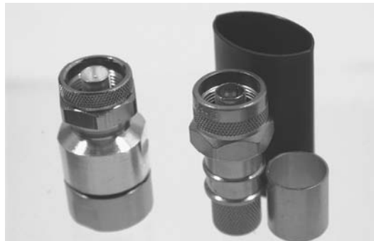
FIGURE 5-25 LMR600 N-Type connector on the right is a crimp-on and the one on the left is an EZ Connector.
