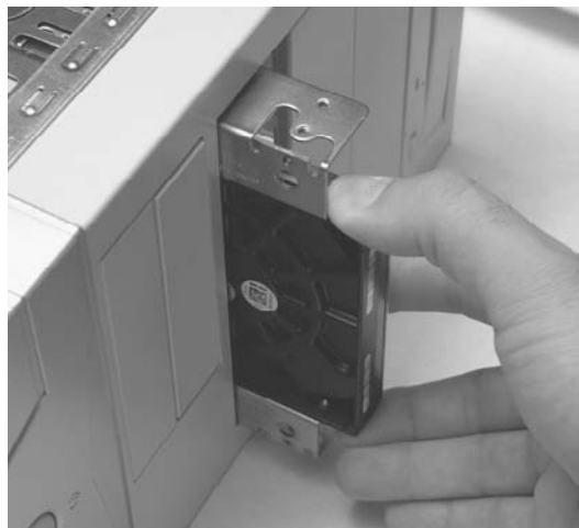
FIGURE 8-13 Adding a 3½" hard drive into a 5¼" DVD drive bay using an adapter.
