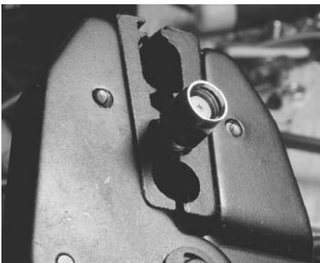
FIGURE 5-24 Have the right size crimping tool or you may damage the connector and/or cable. Once completed, weatherize the end with rubber or electrical tape.
