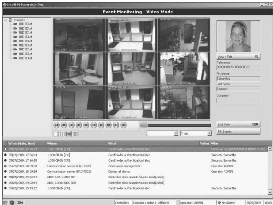
FIGURE 10-1 The Intelli-M Supervisor software interface incorporates video surveillance and access control using an IP-based solution.
