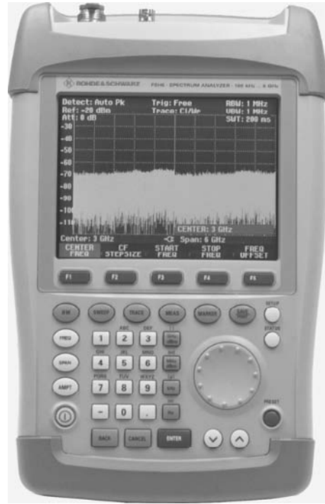
FIGURE 6-11 The Rode & Schwarz FSH6 Spectrum analyzer can detect any RF frequency up to 6 GHz.
