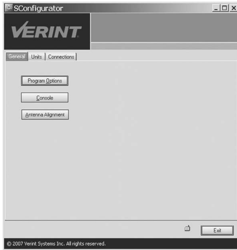
FIGURE 3-19 Verint's proprietary SConfigurator software is one way to discover a Verint device on the network and configure it. Most of the high-end digital video encoder manufacturers provide similar installation software.
