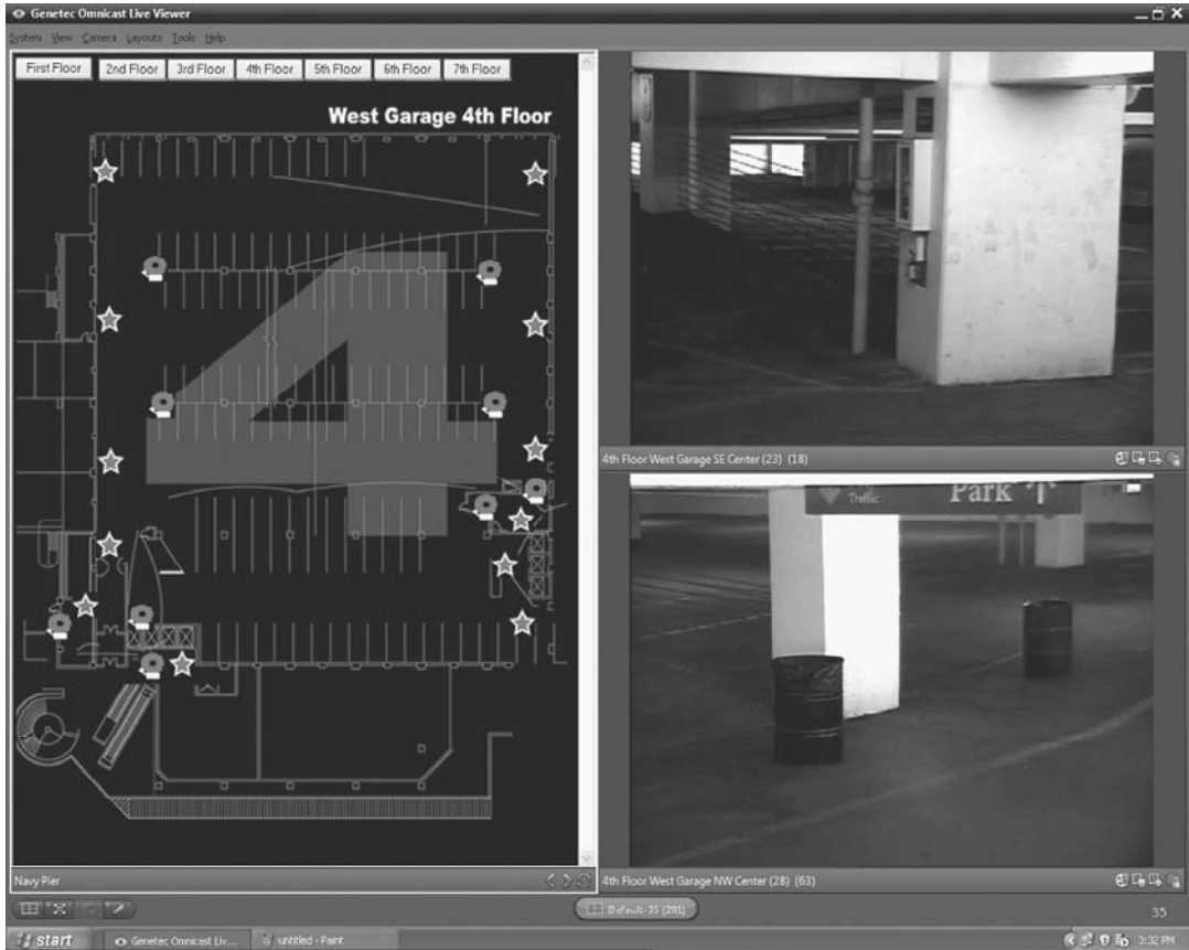
FIGURE 10-12 Parking garage fourth floor map with locations of each camera and panic call box (image courtesy of Navy Pier, Chicago).
