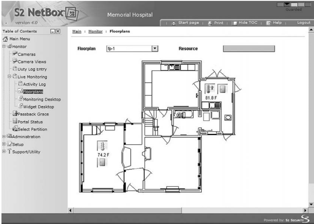
FIGURE 10-15 S2 NetBox Solution can use a map to monitor employee locations, room temperature, and even alarms.
