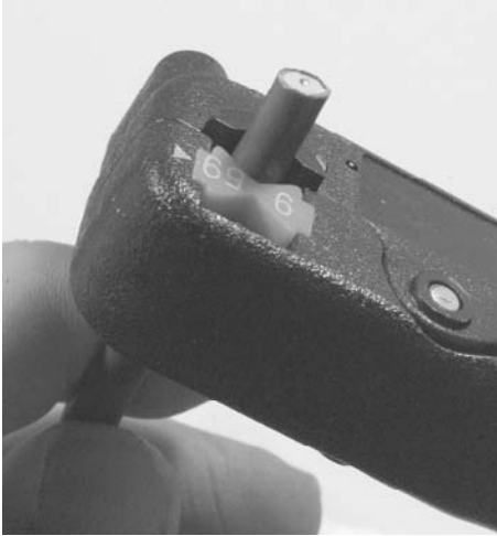
FIGURE 5-20 Use an LMR195/RG58 stripping tool to begin termination (this tool also works well with Ethernet cables).
