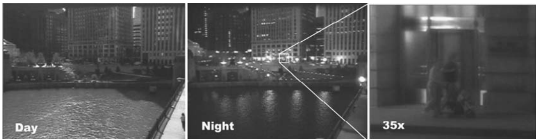
FIGURE 3-13 The urban environment makes it easy to see in the dark. This is a high-performance professional PTZ security camera during the day and then night, zooming into the entrance of the far building.
