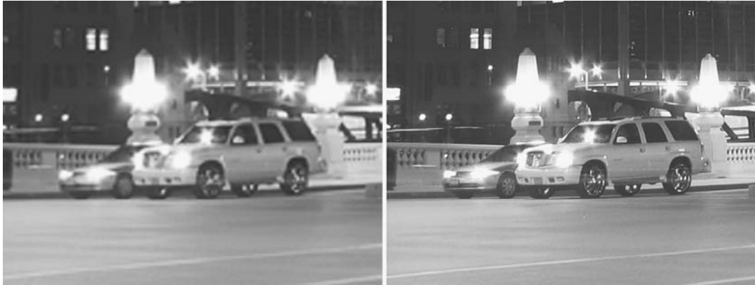
FIGURE 2-6 (Left) Printed screen shot of a 4CIF high-resolution analog video security camera connected to a digital video encoder (704 × 480). (Right) Printed screen shot of the same area of coverage, using a megapixel camera.
