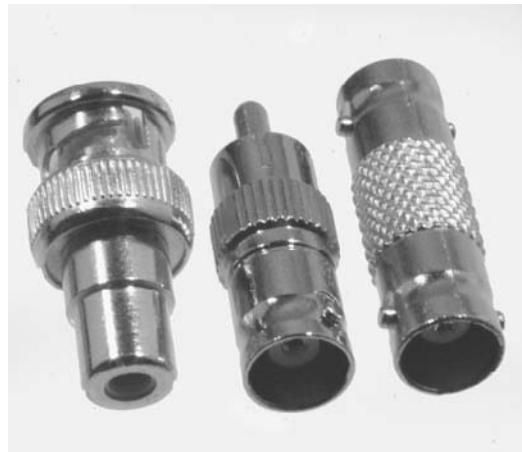
FIGURE 3-25 Video cable adapters from left to right: RCA composite female to BNC male, BNC female to RCA composite male, and a female-to-female BNC coupler to extend a BNC cable using another BNC cable.
