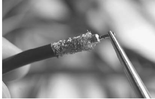
FIGURE 5-21 LMR195, RG58 cable SMA connectors are small and a challenge to handle.
