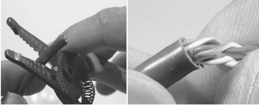
FIGURE 3-27 We all take shortcuts, but avoid damaging the twisted pair when stripping.
