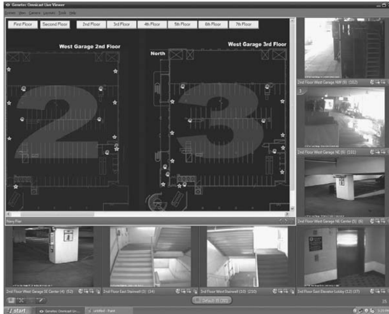
FIGURE 1-9 Maps of each floor were added to help locate the nearest camera.
