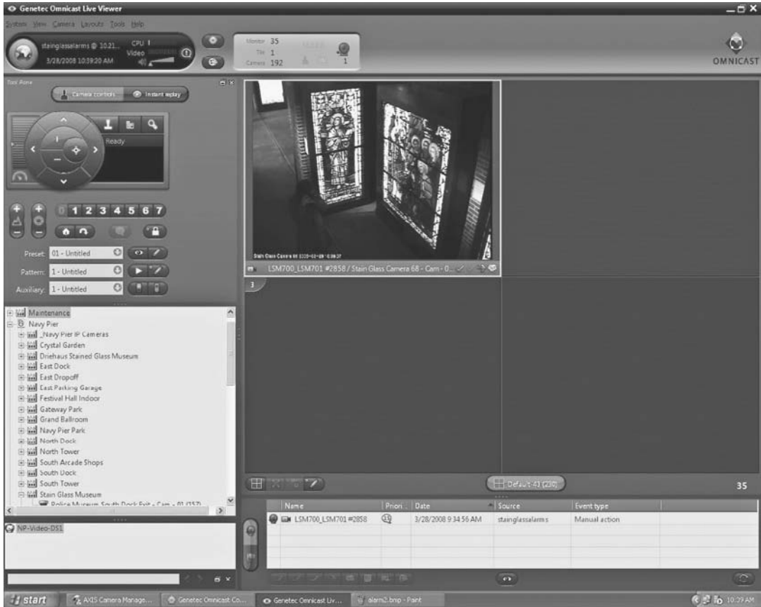
FIGURE 10-10 The Smith Museum of Stained Glass Windows is wired with sensors linked to the video surveillance cameras (image courtesy of Navy Pier, Chicago).
