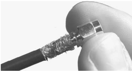
FIGURE 5-22 The SMA crimp-on connector slides underneath the braided insulation.
