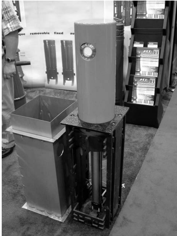
FIGURE 20.40 A view of the mechanics and pneumatics of a retractable bollard. The bollard is dropped into the steel casing and submerged below the ground. The bollard is shown in an extended position.
