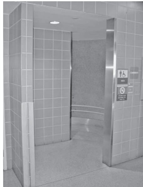
FIGURE 18.26 A lazy S design bathroom door entry.
