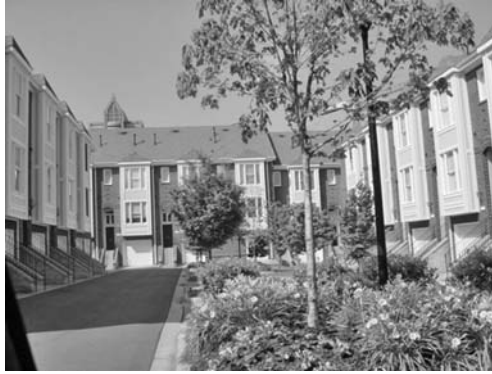
FIGURE 17.27 This picture demonstrates a courtyard concept. These walkup apartments are built above their garages and have good natural surveillance of their common area spaces. CPTED lighting and landscaping facilitate good surveillance.
