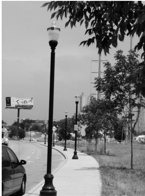
FIGURE 21.33 This street lighting fixture along a park shines light upward and produces light pollution and light trespass.
