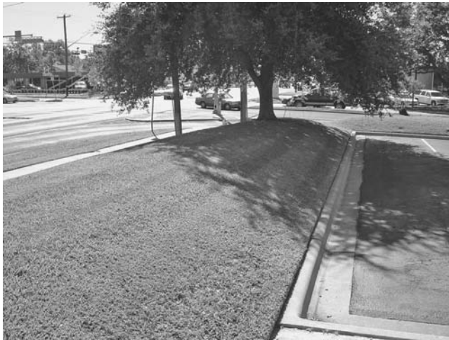
FIGURE 20.11 The berm is almost four feet high and screens the cars from street, but makes natural surveillance from the street by police or passersby almost impossible.
