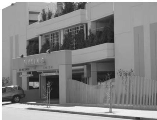
FIGURE 24.9 This garage has a well-defined entrance and a clear and aesthetically pleasing perimeter that directs cars and people to the designated points.
