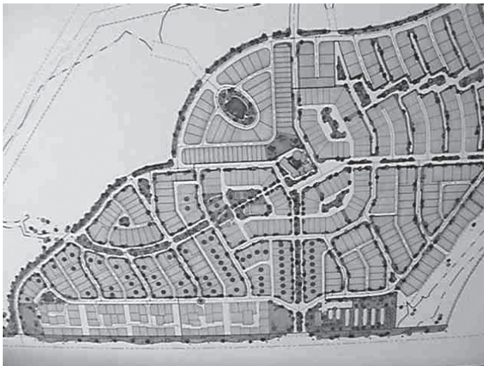
FIGURE 17.7 Civano, Arizona—a New Urbanist town. Their site plan shows the mixed-use zoning and the radial nature of the community.
