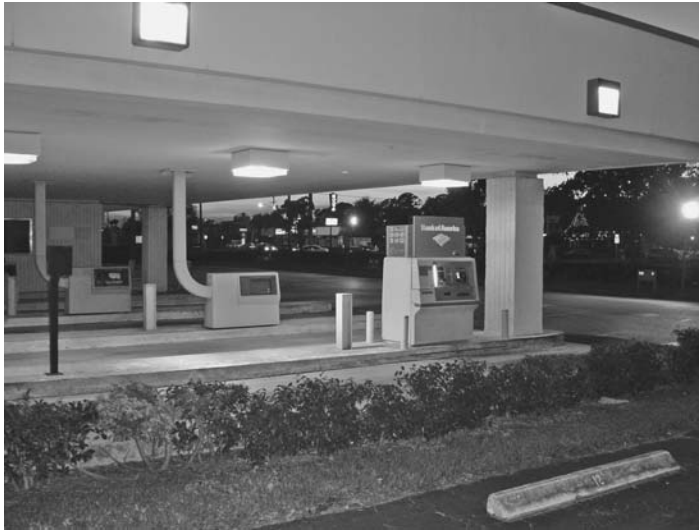
FIGURE 19.7 Plantings must be trimmed low to prevent hiding spaces for ambush of customers.
