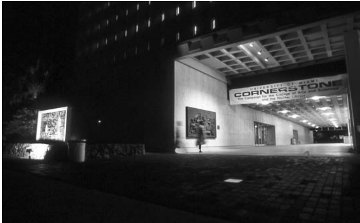
FIGURE 22.22 This picture illustrates the transition of spaces from dark to light and the deep shadow that happens from too drastic a transition.
