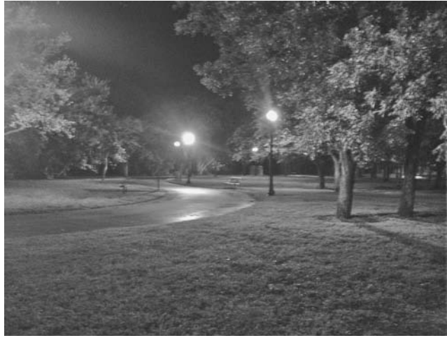
FIGURE 21.32 Globe-style luminaries cast light up and not just on the pathways of this park in Miami Beach, which is problematic for turtle nesting.
