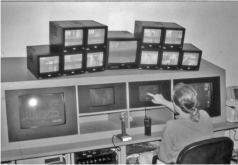
FIGURE 5.1 An example of an ergonomically incorrect design, with monitors too small and too far away to be effective.
