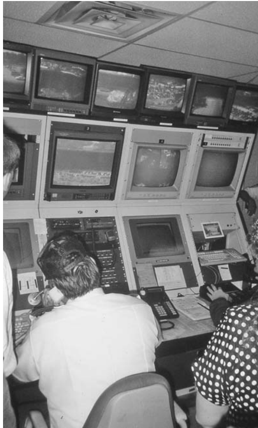
FIGURE 5.3 This control room is out of control. Human factors was not a design consideration here.
