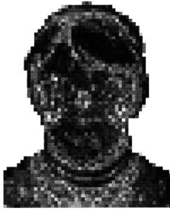
Figure 1.3 Identification based on facial thermograms [1]. The image is obtained by sensing the infrared radiations from the face of a person. The graylevel at each pixel is characteristic of the magnitude of the radiation.
