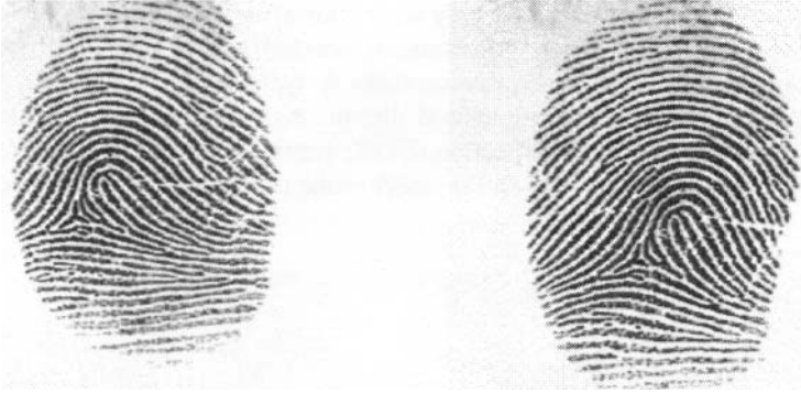
Figure 1.23 Impressions of a finger captured by exerting different (magnitude/direction) forces on the finger during fingerprint acquisition results in a significant non-homogenous distortion of the ridge structures; consequently, the fingerprints are difficult to match.
