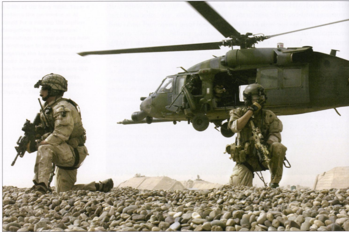
USAF Para Rescue Jumpers maintain security at an HLZ. The ARSOC HH-60 Pave Hawk features a mid-air refuelling probe, and has .50cal M2s in the door-gunner hatches. (Courtesy USSOCOM)
