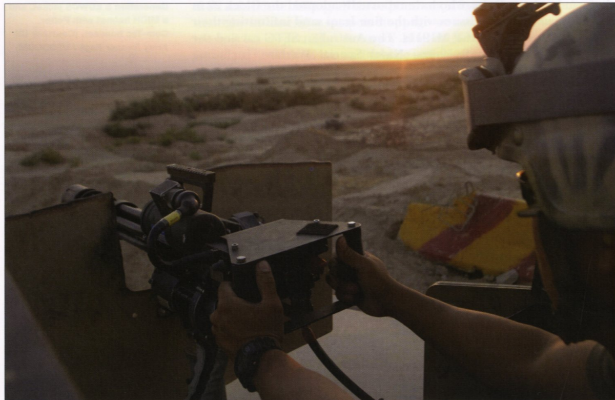
An alternative to the usual .50cal M2 or 40mm Mk19 AGL in the top turret ring of GMVs is a minigun; here a 7.62x51mm M134 is being test-fired at an Iraqi range. (Courtesy US Navy; photo Mass Comm Spec 2nd Class Christopher Perez)
