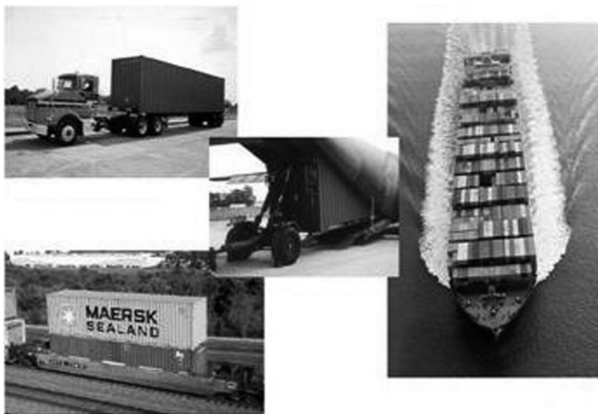
FIGURE 9.7 Methods of Intermodal Transport
