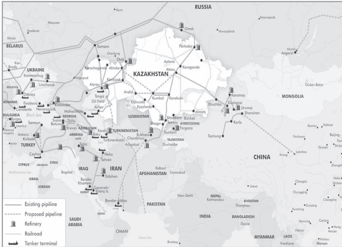
Figure 8.1 Oil Pipelines and Infrastructure of the Caspian Region Source: Energy Information Administration
