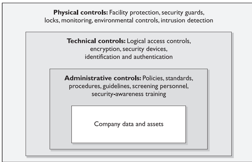
Figure 3-1 Administrative, technical, and physical controls should work in a synergistic manner to protect a company's assets.
