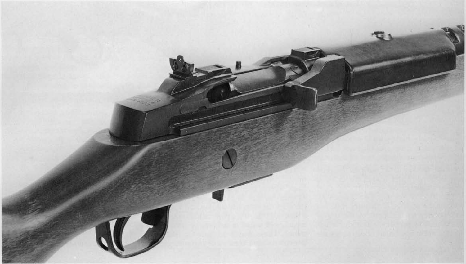
Above: Close up right view of the breech of the Ruger Mini-14 .223 caliber rifle. Below: The same rifle field-stripped.
