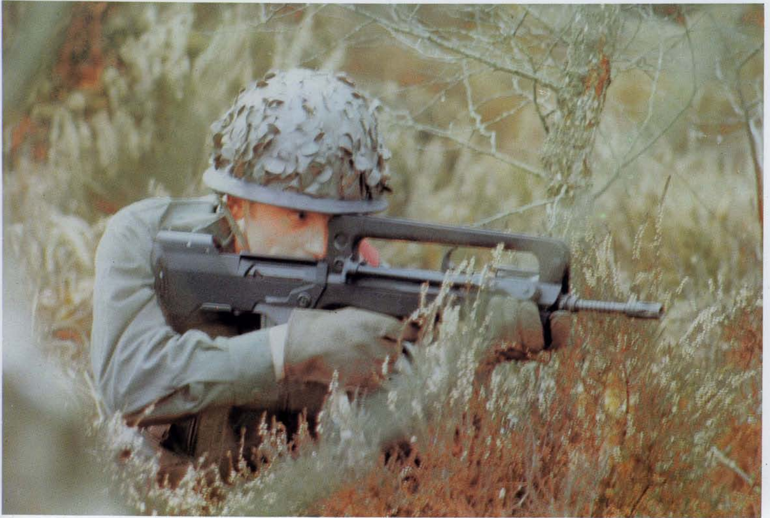
Above: A REXIM submachine gun. Below: A French infantryman takes aim with his FAMAS 'Trumpet' assault rifle. Note the folded bipod and the long protected sight lying within the carrying handle. Right: A Steyr MP1 69 machine pistol
