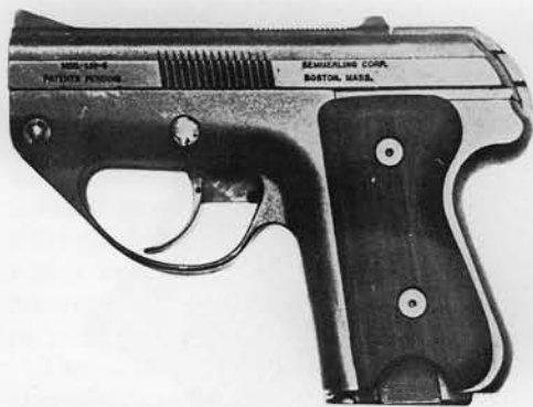
The Semmerling LM-4 pistol, a hand-actuated repeater.
