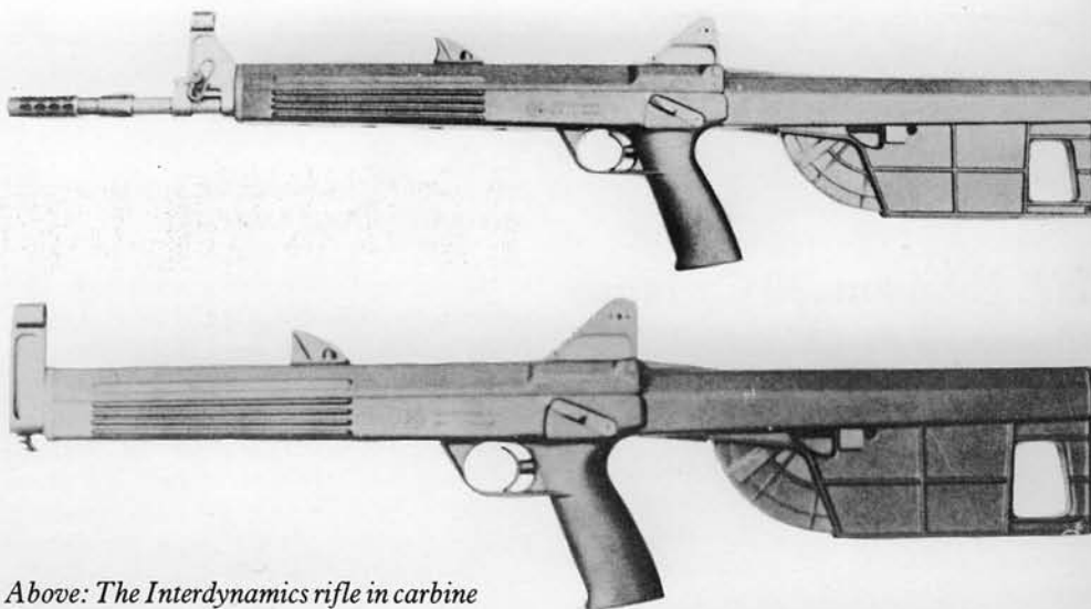
Top: The Swedish Interdynamics rimfire military rifle; the semi-circular protrusion in the front of the butt is the magazine.
