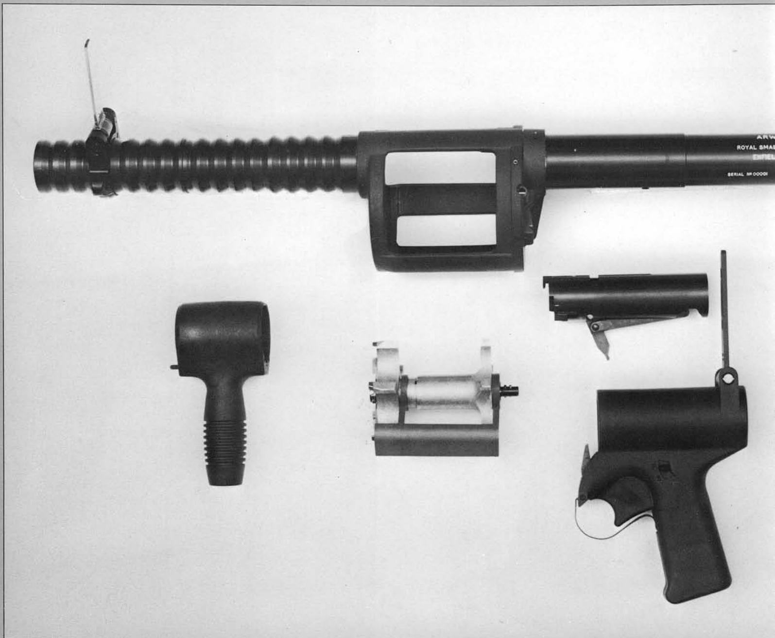
The ARWEN reduced to its component parts; barrel on the left, action body on the right, cylinder housing in the center. The bolt is above the pistol grip and the five-shot sprocket feed is detached. The entire weapon is of alloy and plastic and is surprisingly light.
