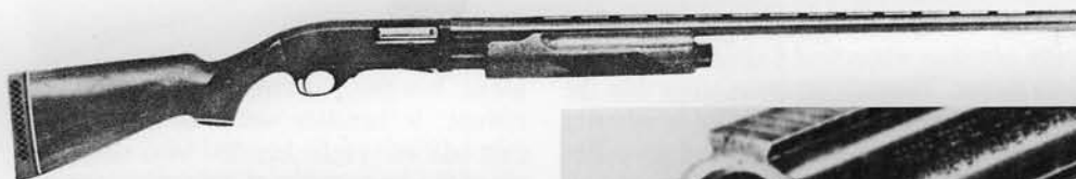
Left: The Smith & Wesson Model 1000P is a pump-action gun, which uses many of the parts of the automatic version.
