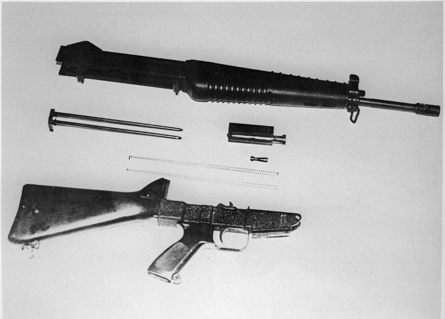
Below: The SAR 80 field-stripped, showing the simple design.
