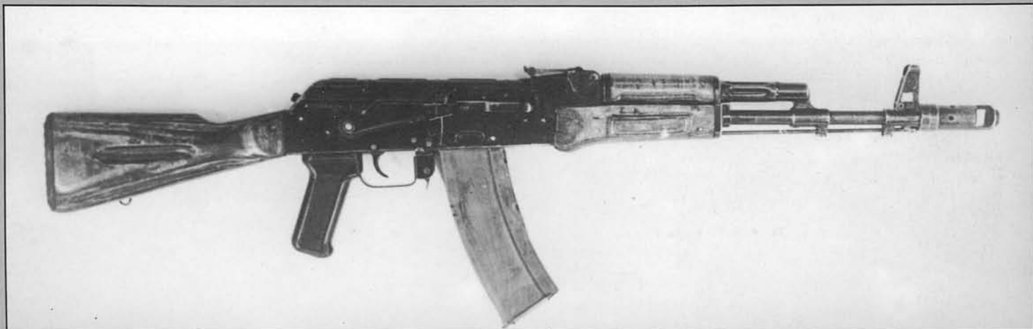
Below: The Soviet AK74 in 5.45mm caliber, currently being used in Afghanistan.
