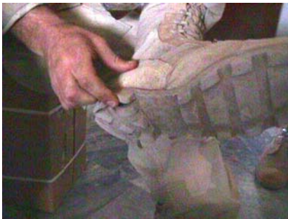
Damaged sole of Desert Combat Boot
