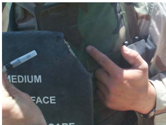
7.62 round glanced edge of SAPI and embedded in OTV
