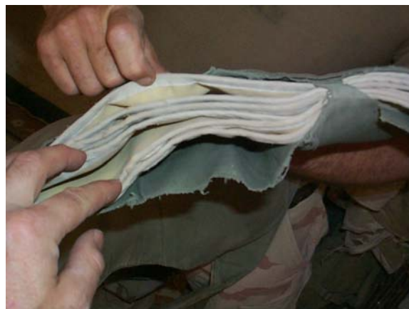
Soldier-modified Spall Vest with 3X protection (6 layers)
