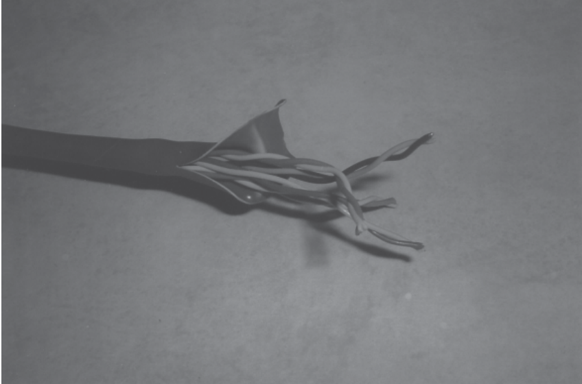
Figure 9-1. Unshielded Twisted Pair Wire. This photo of what is called CAT 5 cable contains four pairs of wires. (Photo by Robert Reid, 2004)
