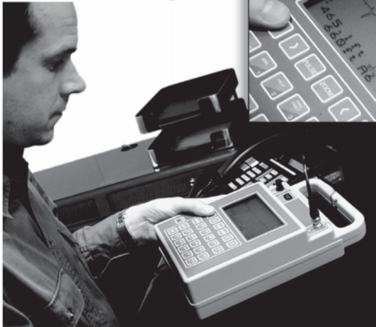
Figure 12-2. Time domain reflectometry. Source: Murray and Associates, Oldwick, NJ.
