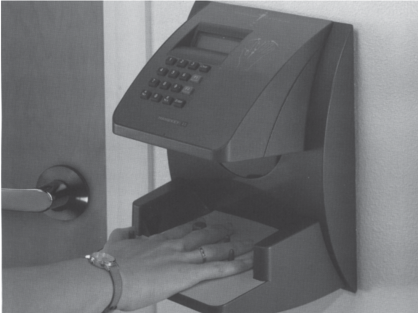
Figure 8-5. Palm reader. Reprinted with permission. IR Safety and Security-Americas Copyright 2003. All Rights Reserved
