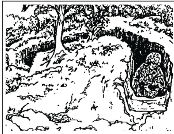
Figure 071-326-5703-4. Fighting position on slope
