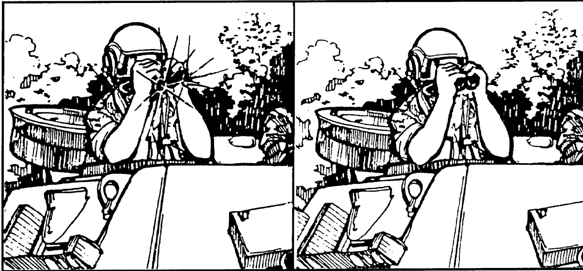
Figure E-1. Shade optics to prevent shine.
