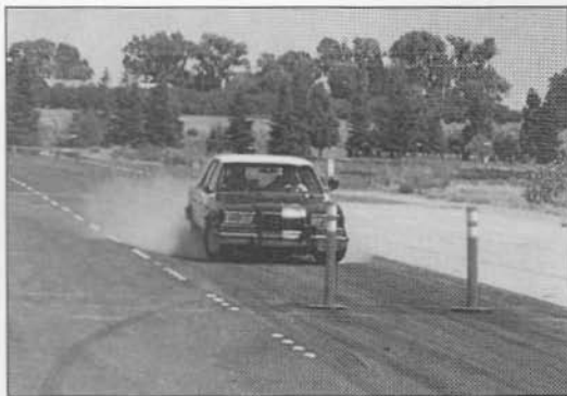
The most common braking error during a panic stop or an accident avoidance is locking the brakes. Larry Hollingsworth
