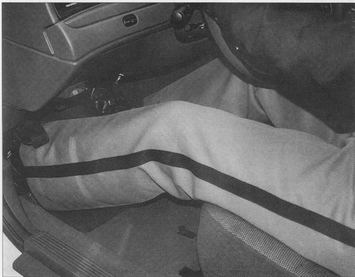
The proper position for the left foot is on the "dead pedal" to the far left of the floorboard. Use the left foot to brace yourself in a nice three-point suspension.
