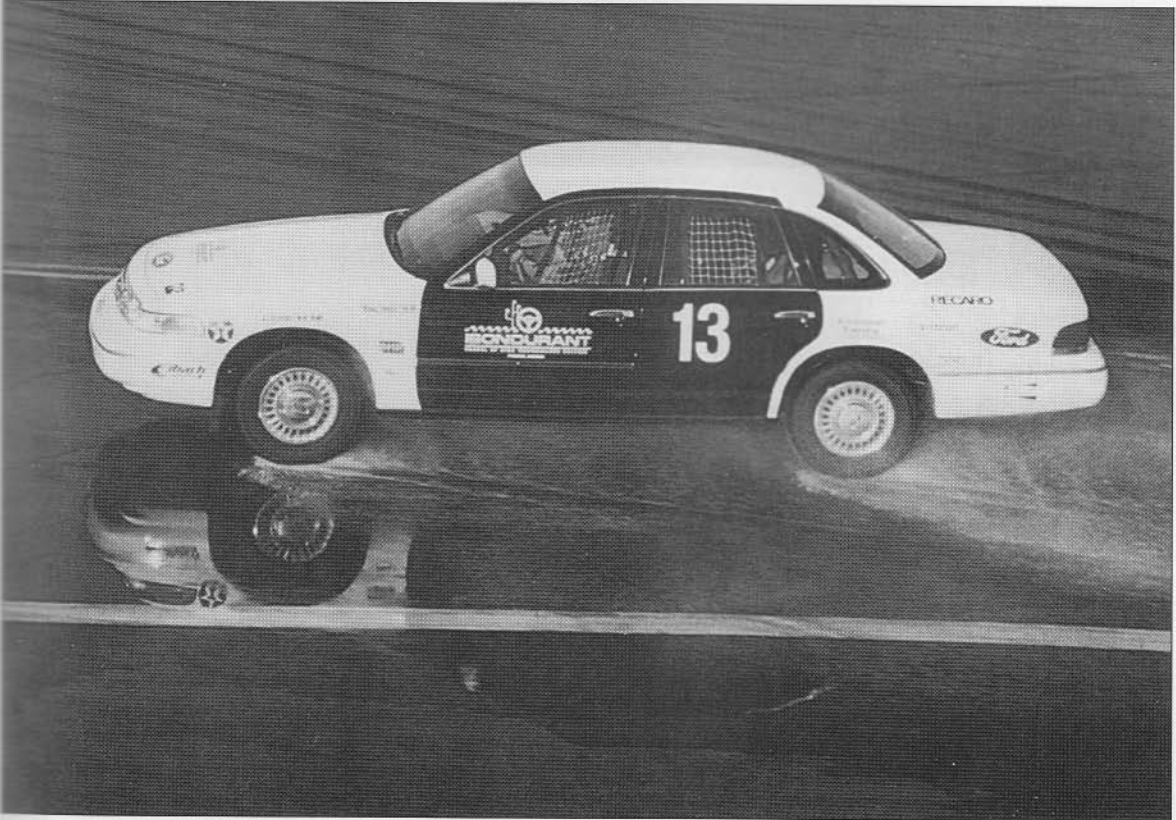
In a car without ABS, or with ABS deactivated, it is easy to lose steering and braking control under wet conditions.
