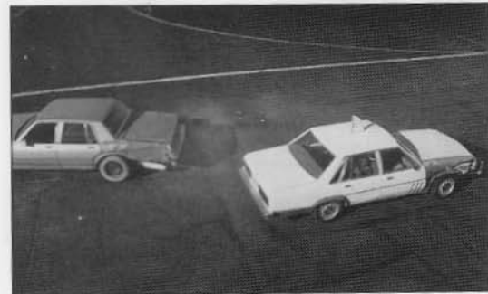
Low-impact speeds work the best for the roadblock ram. Low impact speeds are least likely to set off an air bag in the police car and are the least likely to shut off the electronic fuel pump. Greg Fresquez
