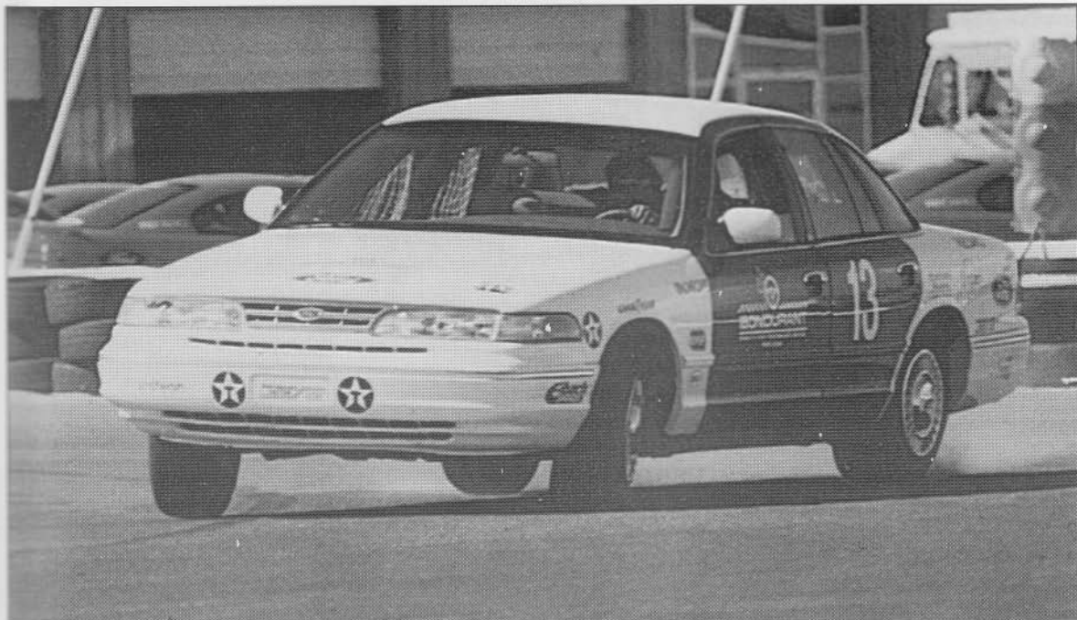
Oversteer occurs when the rear tires lose traction, and the rear of the car swings to the outside of the corner. This causes the front end to point "more" in the corner than the driver wants. It "over" steers. Rick Scuteri
