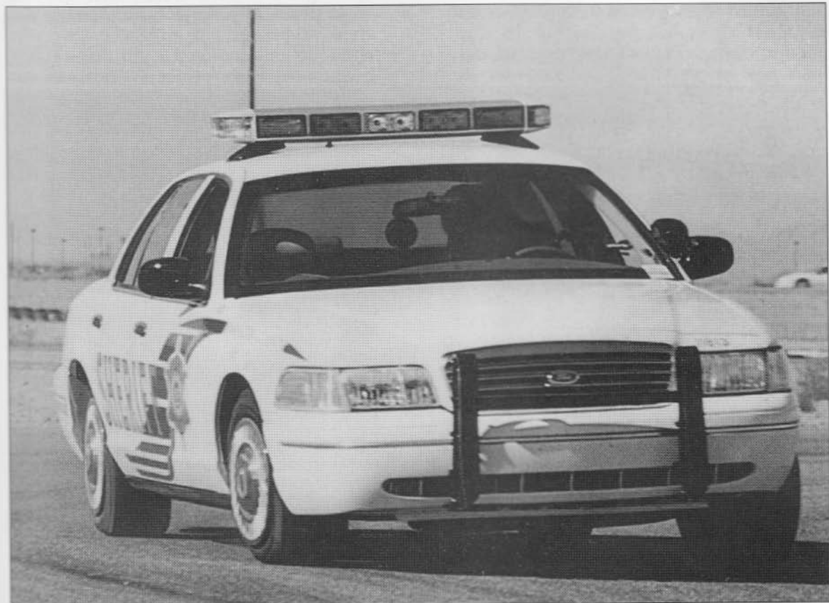
Here is the same police car going around a curve at maximum adhesion. Even the stiffly sprung Ford Police Interceptor has rolled slightly to the outside. A great deal of weight is on the outside front tire. Note how much the tire is rolled under, compared to the car at rest.
