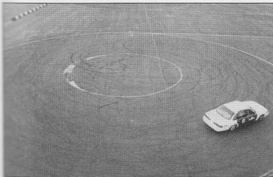
With less weight, smaller tire patches, and less traction on the front tires, the police car pushes to the outside of the circle. The steering wheel has not moved.
