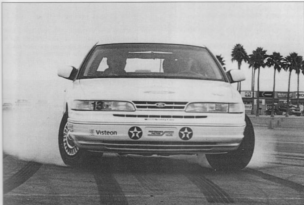
The driver can turn the wheels all the way left or right, but with locked brakes, the car goes straight.
