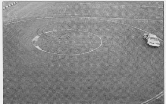
The police car has moved from the inner circle to the outer circle simply due to weight transfer. As the officer lifts off the gas, the weight will shift back to the front and the car will turn hard into the inner circle again.
