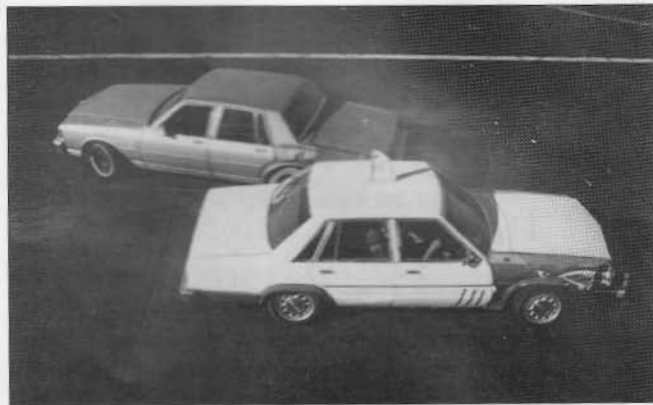
The ramming vehicle easily pushes the blocking vehicle aside, leaving a completely open lane. The ramming vehicle is not tossed off course at all. Greg Fresquez
