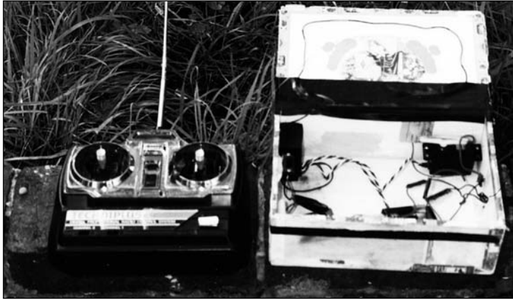
Remote Control Device. Remote control unit with the device installed in a cigar box. The range of such a device, whilst only measured in 10's of metres, can still make an effective terrorist weapon.
