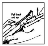
Figure 071-311-2025-10. Removing the bolt carrier and bolt
