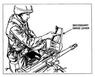
Figure 071-030-0005-3. Indexing the feed slide assembly
