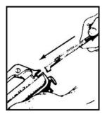
Figure 071-311-2025-32. Placing the charging handle in the receiver
