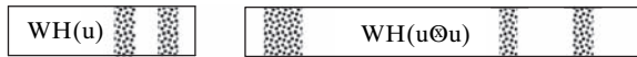
Figure 11.2. The \mathbf{PCP} proof that a set of quadratic equations is satisfiable consists of \text{WH}(u) and \text{WH}(u \otimes u) for some vector u . The verifier first checks that the proof is close to having this form and then uses the local decoder of the Walsh-Hadamard code to ensure that u is a solution for the quadratic equation instance. The dotted areas represent corrupted coordinates.
