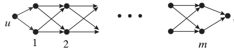
Figure 17.1. Reducing Ham to #CYCLE: by replacing every edge in G with the above gadget to obtain G' , every simple cycle of length \ell in G becomes (2^m)^\ell simple cycles in G' .
