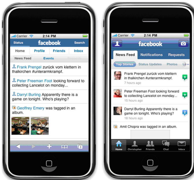
Figure C.2 Spot the difference: the Facebook web application on the left and the Facebook native application. The web application lacks certain features, such as access to the camera and photo library.
