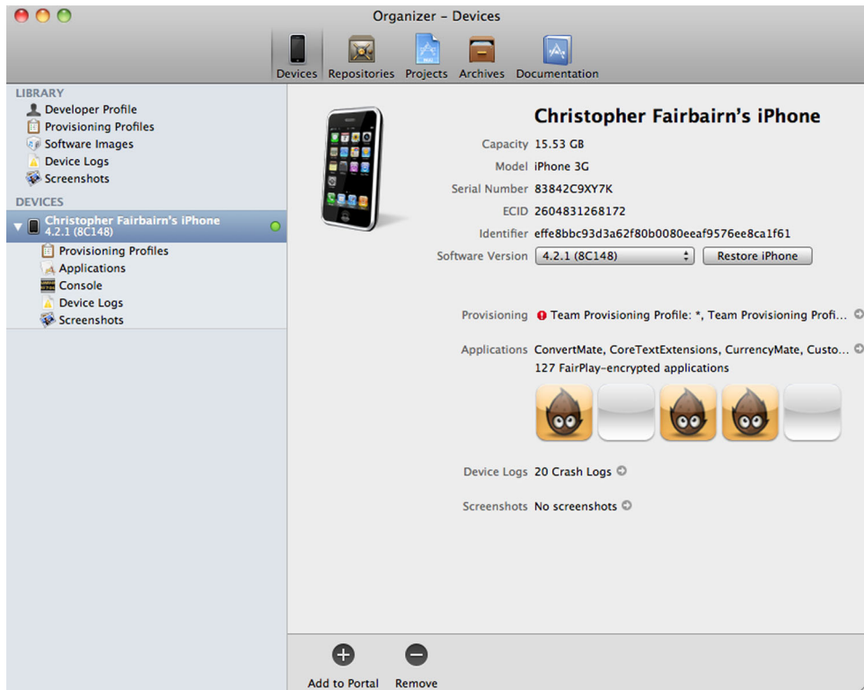
Figure 14.2 The Xcode Organizer window showing a list of connected iOS devices. Using the various tabs, you can control different aspects of your connected device, such as installing and uninstalling applications, maintaining provisioning profiles, capturing screenshots, and reviewing application crashes and log files.
