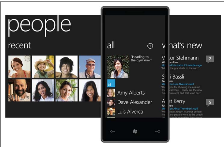
Figure 3-3. The panoramic UI design pattern shows a bit of the following content at the right, and the user can scroll the whole screen using his fingers. Here is a Windows Phone 7 screen.
