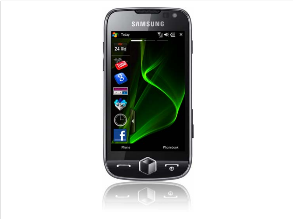
Figure 1-10. The Samsung Omnia is a Windows Mobile 6.5 device. The operating system is very friendly for desktop Windows users, featuring the Start menu and a very similar user interface.
