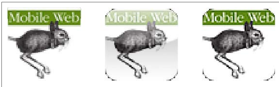
Figure 6-1. The original 57×57-pixel iPhone icon file, the final appearance once the website has been added to the home screen, and the icon using the precomposed meta tag.
