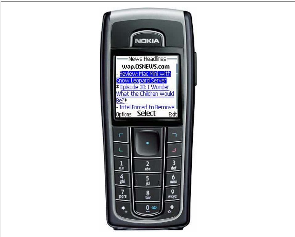
Figure 5-1. A typical WML document contains just text, links, and maybe some little image. It is always focus-based and optionally can execute WMLScript code, but that is very rarely used.
