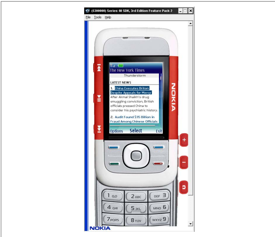
Figure 4-5. Here is a focus-based navigator over a Nokia S40 emulator. If you use File→Open , you must type http:// first.
