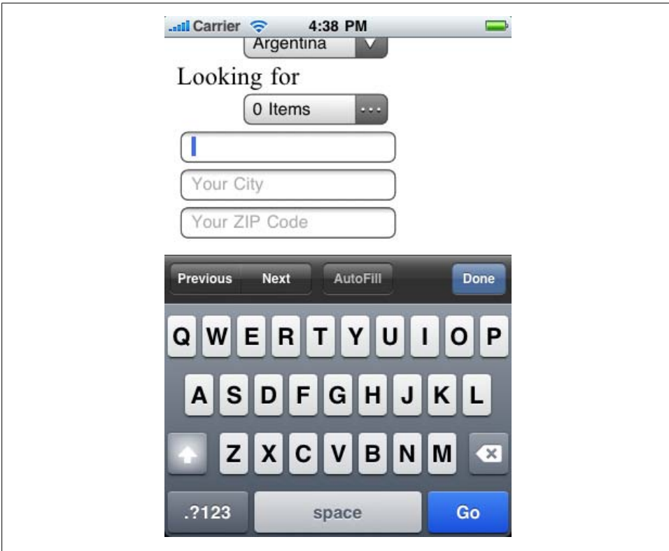
Figure 6-14. The placeholder is the gray descriptive text inside the text box that is automatically deleted when the user begins typing a value in the box.
