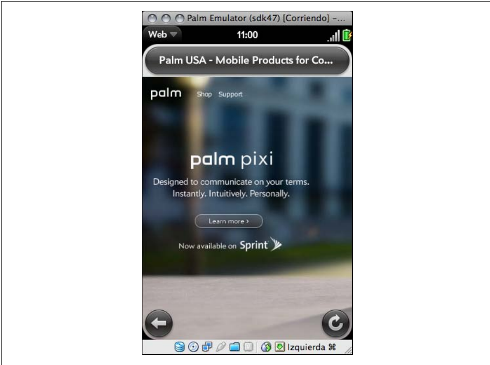
Figure 4-8. The webOS emulator doesn't have an onscreen keyboard, so you need to learn the shortcuts to emulate keypresses.
