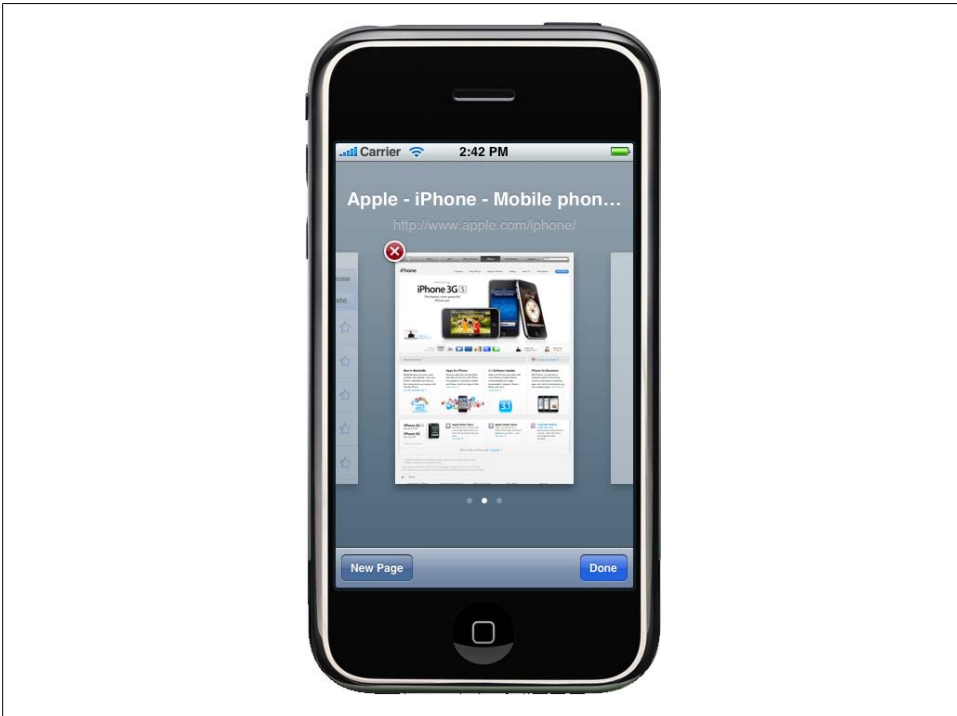
Figure 2-5. The iPhone browser has multiwindow support that allows the user to maintain up to eight different websites open at the same time. Android and webOS have similar features.
