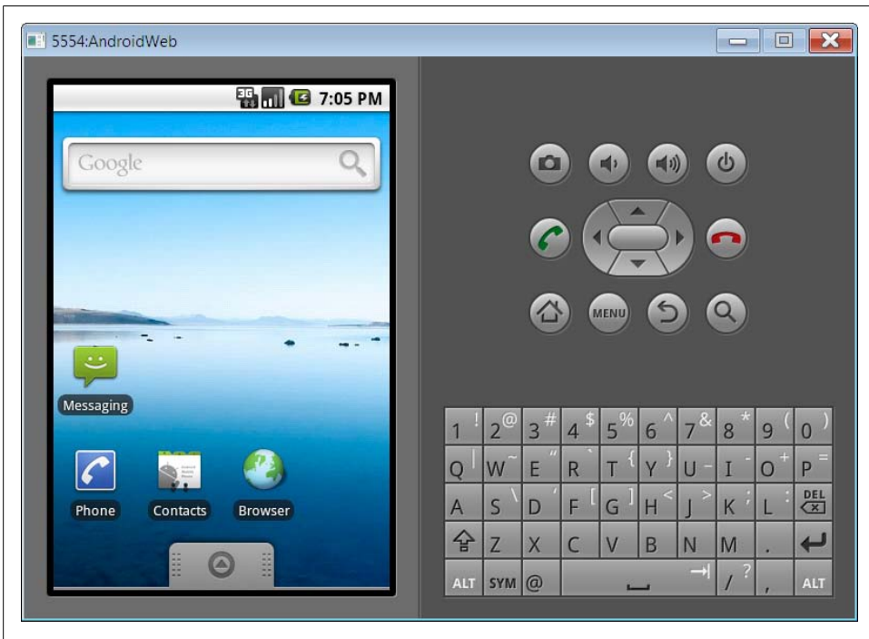
Figure 4-4. At this point, you can open the browser as if you were on a touch-enabled Android device. You can use the mouse over the emulator’s screen to emulate the user’s gestures.
