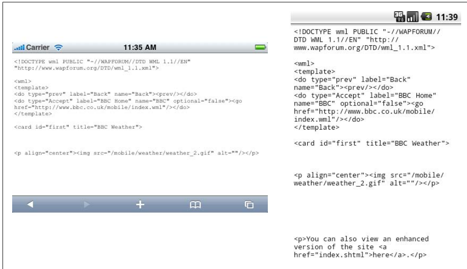
Figure 5-2. Both the iPhone and Android browsers show the WML source code instead of rendering it.
