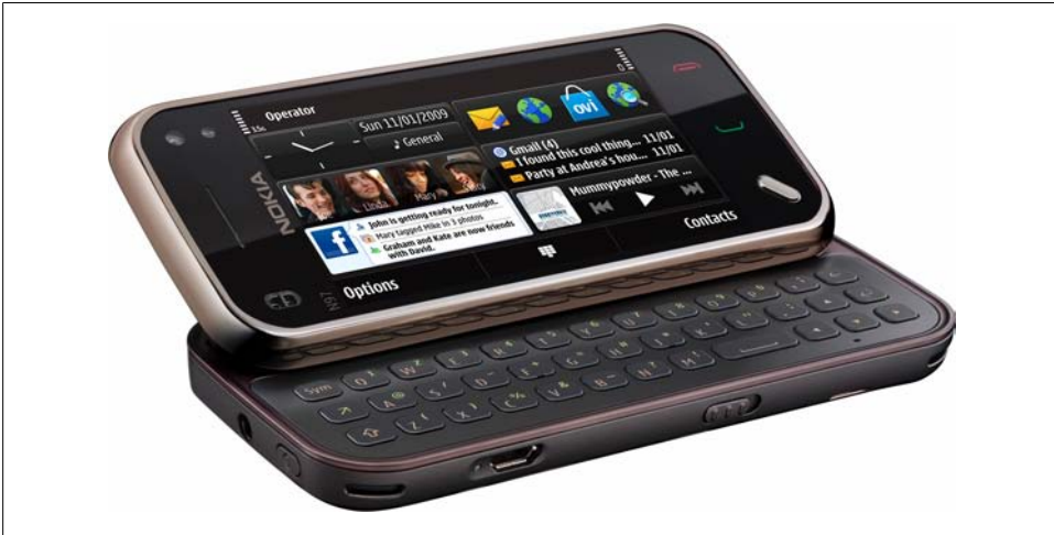
Figure 1-5. The Nokia N97 mini has a full slider QWERTY keyboard and, when closed, an onscreen touch keyboard.
