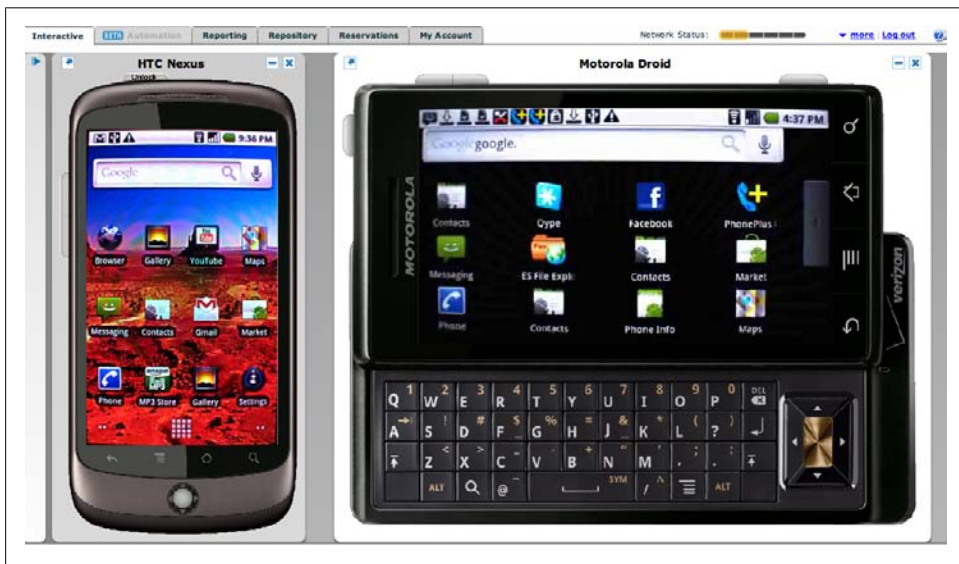
Figure 13-4. With Perfecto Mobile you can manage real phones (here, a Nexus One and a Motorola Droid) with a Flash-compatible browser. The images are from cameras pointing at the devices.
