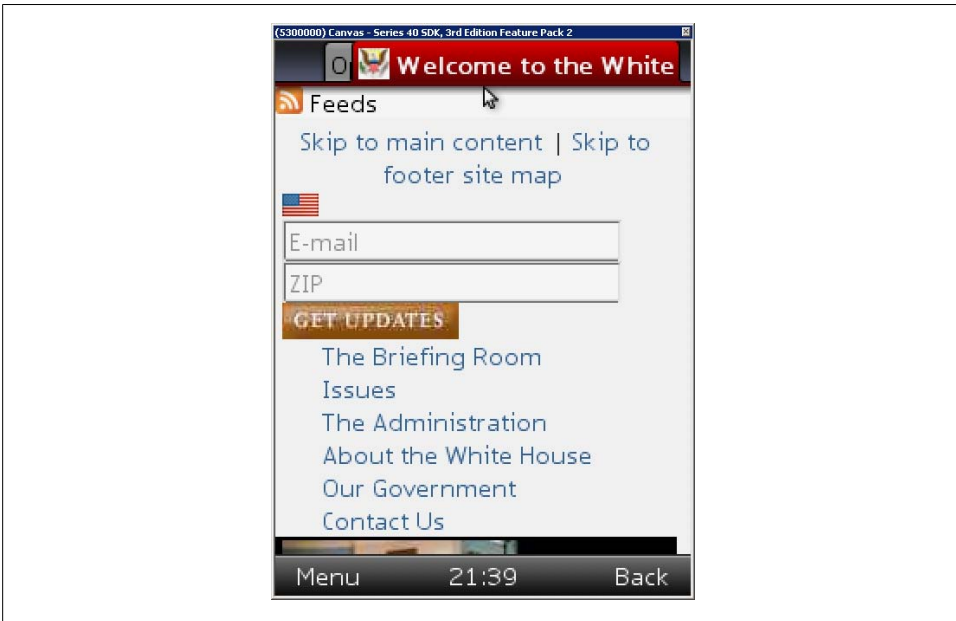
Figure 2-4. The same website as in Figure 2-3 viewed with Opera Mini “Mobile View,” a reflow engine that autodetects navigation bars, content zones, and footers and shows us a one-column view of the site.
