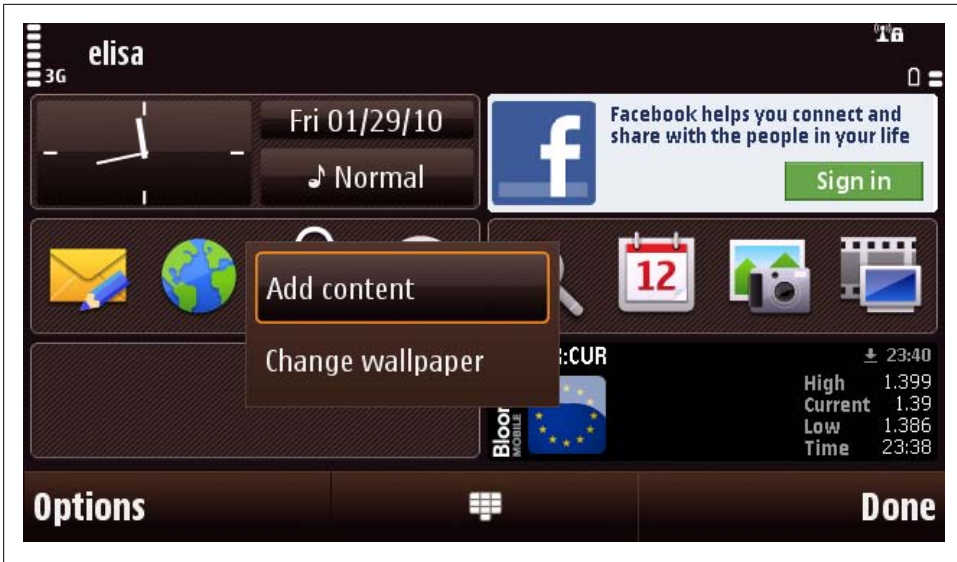
Figure 12-3. With the MiniView, users can add our mobile web content to their home screens. Using JavaScript, the information displayed in the widget can be updated on a regular basis.
