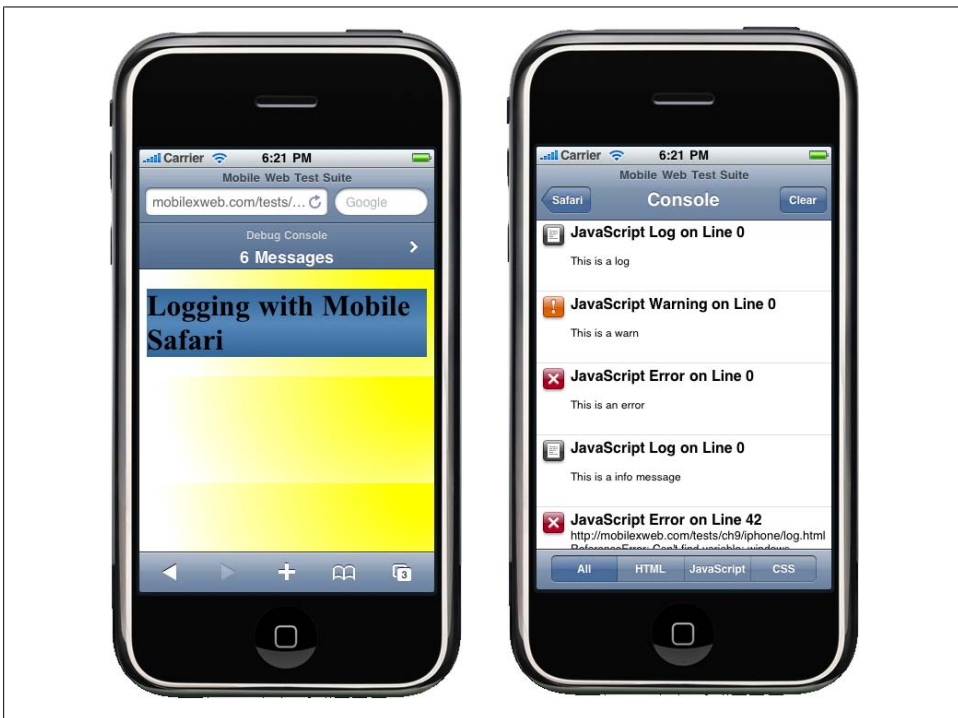
Figure 13-9. When you activate the debug console you will see the console toolbar (left), which you can click on to access a details list (right).
