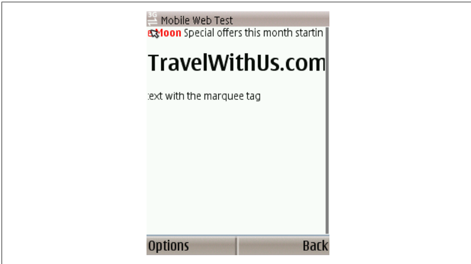
Figure 5-9. A Nokia N95 showing a marquee animation in progress using standard WAP CSS.
