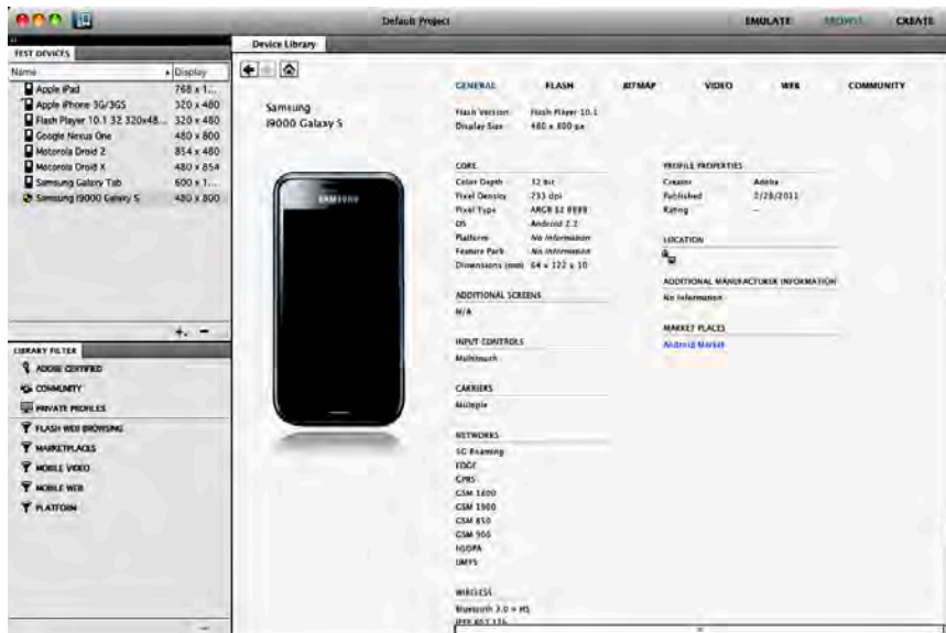
Figure 9-4. Click and drag the device to the Test Devices panel to add it to the devices to test against
