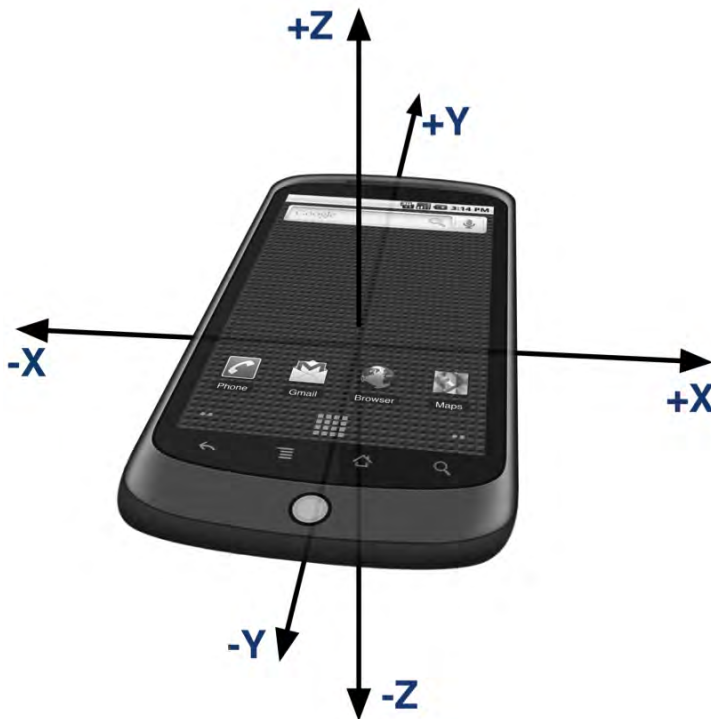
Figure 7–8. The accelerometer axes of an Android phone
