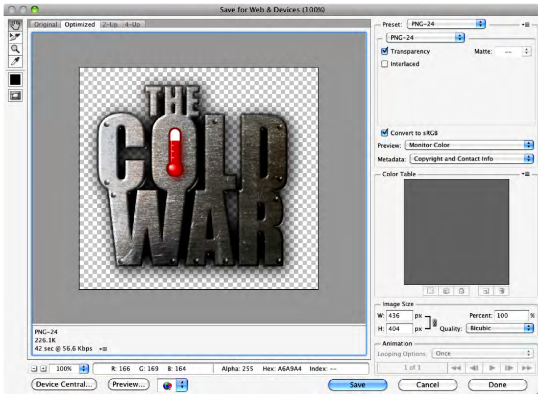
Figure 9-11. Exporting a graphic from Photoshop using File > Save for Web and Devices
