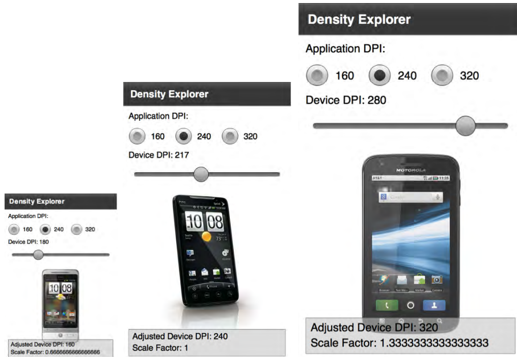
Figure 2-4. Side-by-side comparison of the Density Explorer when run on a device classified as 160 dpi (left), 240 dpi (center), and 320 dpi (right)
