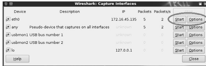
FIGURE 4.17 Wireshark Capture Interfaces Window.
