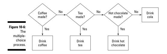
Effectively, this diagram shows several single-process diagrams in a row. Visual Basic 2005 provides you with a structure that handles this kind of situation. A good software design takes advantage of as much of the language in question as possible.
