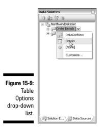
Change the Orders table to a Details view. It is used to create a detail type form — one that easily allows the user to view and change data. Then drag the table to the form, and the Details view is created for you, as shown in Figure 15-10.
