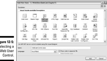
Figure 12-5: Selecting a Web User The process for developing a user control is just like the process for developing a Web Forms page. Drag controls to the screen and double-click to add code to the control. To add your new control to a Web page, just drag the ASCX file to the ASPX page in Design View.
