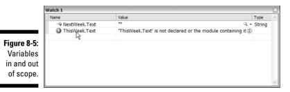
The Watch window is a great way to watch whole objects, rather than just values in variables. Collections, such as arrays and datasets, often have a wide variety of properties and values that you need to check on every break. The Watch window provides a simple method for a structured check on values.
