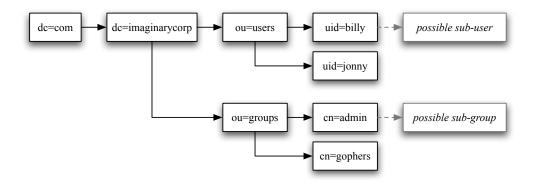
Figure 7-1. LDAP schema section for ImaginaryCorp
