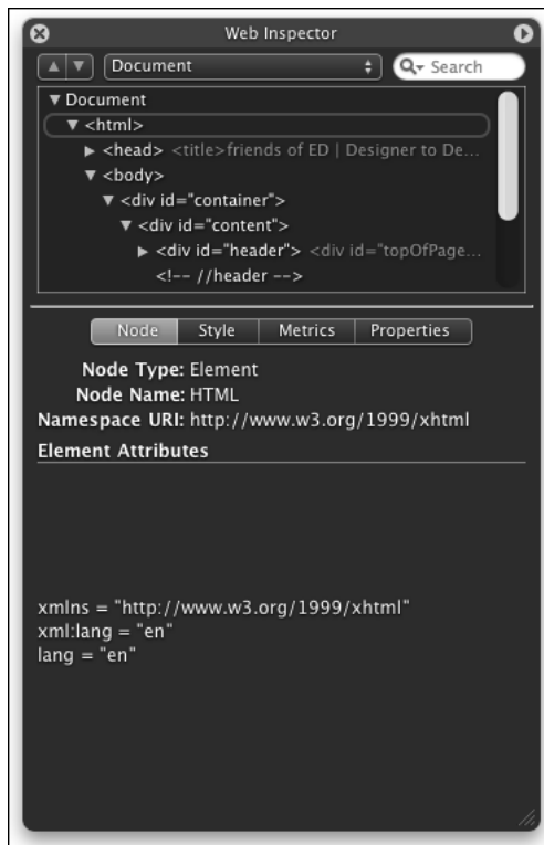
Figure 7-1. In the DOM, a web page is shown as a hierarchical structure, or “tree,” of elements (called nodes in DOM-speak).
