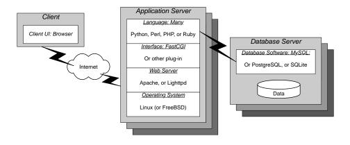
Figure 5.2: Typical LAMP deployments use simple, shared-nothing architectures
