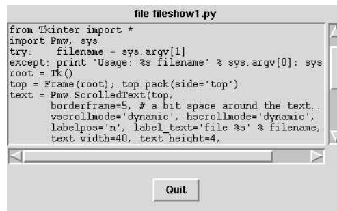
Fig. 6.23. Same GUI as in Figure 6.22, but the text widget is now allowed to expand in size as the main window is enlarged.
