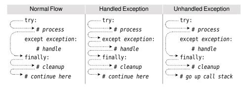
Figure 4.2 Try ... except ... finally control flows
