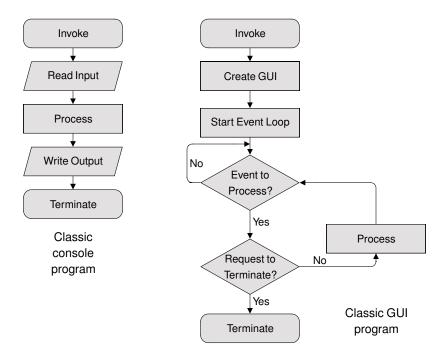
Figure 15.1 Console programs versus GUI programs
