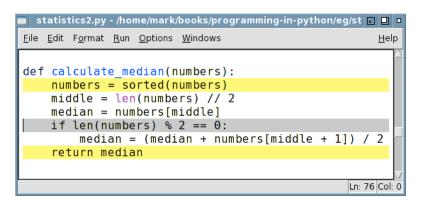
Figure 9.2 An IDLE code editing window during debugging
