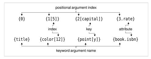
Figure 2.5 Annotated format specifier field name examples
