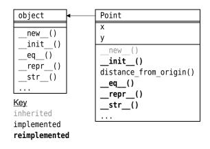
Figure 6.2 The Point class's inheritance hierarchy
