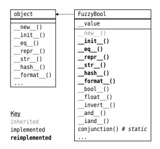
Figure 6.4 The FuzzyBool class's inheritance hierarchy
