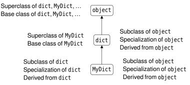
Figure 6.1 Some object-oriented inheritance terminology
