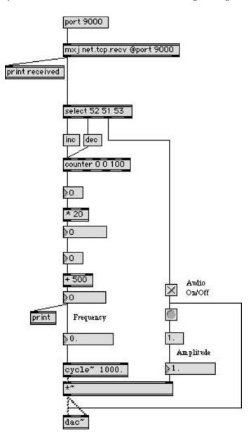
Figure 11.11 Max/MSP patch using TCP port
