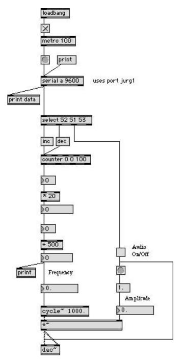
Figure 11.8 Max/MSP patch using Bluetooth
