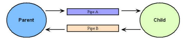
Here we see two processes which I've called Parent and Child, for reasons that will become apparent shortly. The Parent can write to Pipe A. and read from Pipe B. The Child can read from Pipe A and write to Pipe B.
