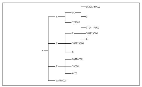
Figure 4-2. Diagram of a suffix tree
