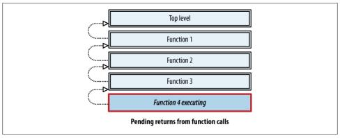
Figure 8-1. Function calling and stack frames
