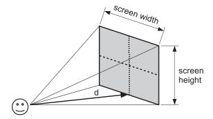
**Figure 8-6.** The viewing distance in a perspective projection
