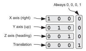
Figure 9-1. Components of a matrix
