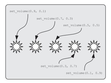
**Figure 10-4.** *Setting the stereo panning of an explosion*
