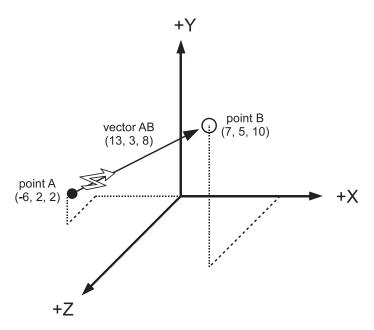
**Figure 8-3.** Calculating a target vector
