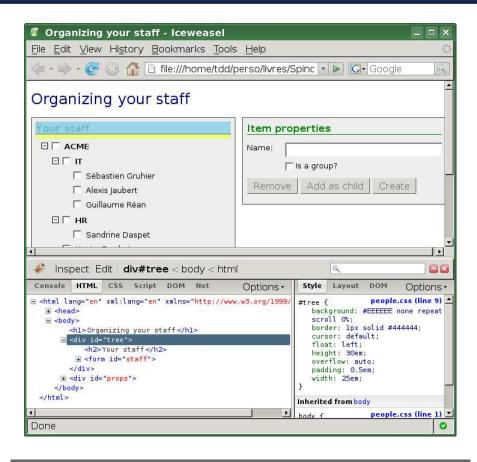
Figure 7.5: Firebug's DOM inspector in action
