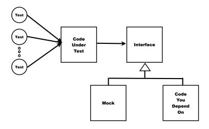
Figure 16.1: Mocking during unit testing
