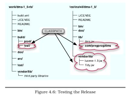
Notice that we overrode the location for production classes using the -Dbuild.prod.dir option. We also overrode the location for vendor libraries using -Dvendor.lib.dir. This means we're running the tests in the release branch directory against the production classes and vendor libraries in the unpacked distribution directory. The compile and compiletests targets did nothing because all the class files are upto-date. We're just using what we already have.
