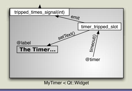
Figure 5.15: Custom Widget with Signals and Slots
