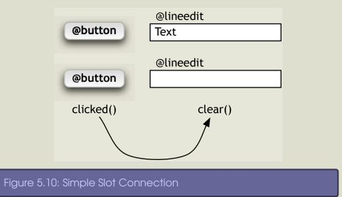
a Qt::LineEdit to clear when a Qt::PushButton is clicked (as seen in Figure 5.10 ).
