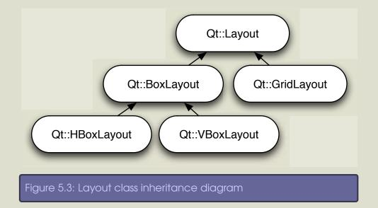
nience classes based on Qt::Layout: Qt::HBoxLayout, Qt::VBoxLayout, and Qt::GridLayout.
