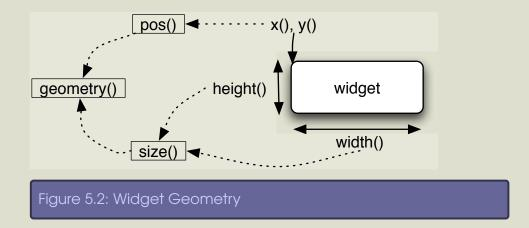
To perform both operations at the same time, use the methods set-Geometry(int x,int y,int h, int w) or setGeometry(Qt::Rect).
