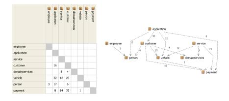
Figure 11.16: The final DSM shows no tangles.
