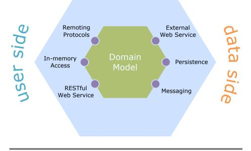
Figure 1.4: The *hexagonal architecture* emphasizes multiple implementations of the different layers.
