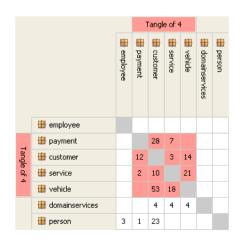
Figure 11.2: The CarServ DSM shows cyclic dependencies.
