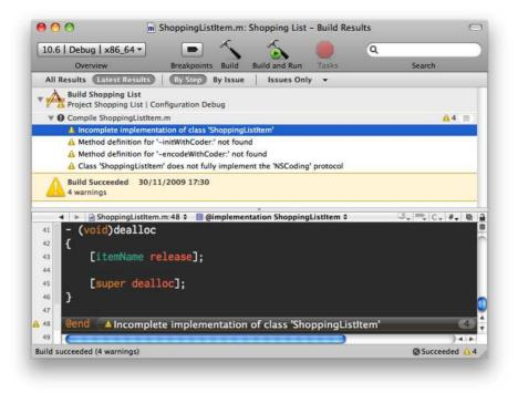
Figure 13.7: Warnings about not fully implementing a protocol
