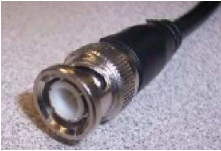
Figure 11.9: A BNC connector on a coaxial cable
