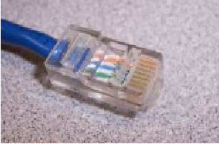
Figure 11.12: An RJ-45 connector at the end of a CAT-5 cable
