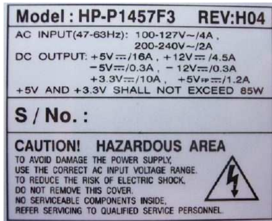
Figure 5.14: Nameplate from a power supply
