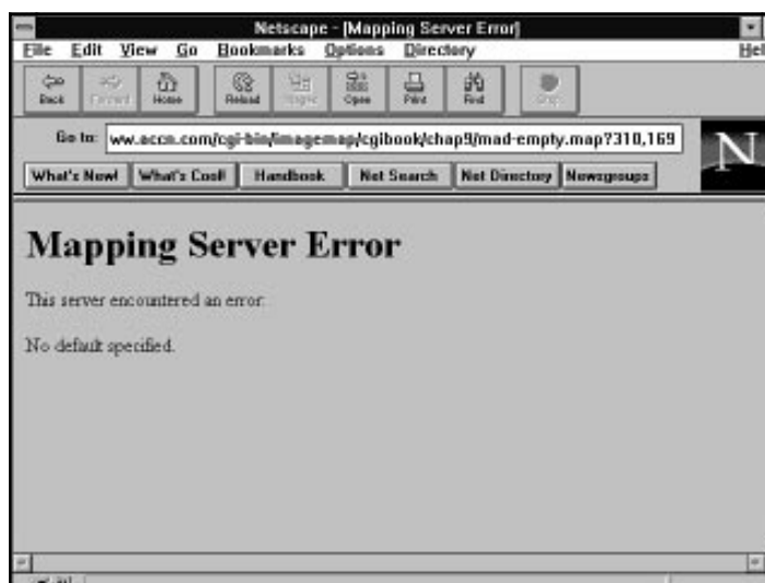
Figure 9.8. The error message sent by the image map program when a default URI is undefined.
