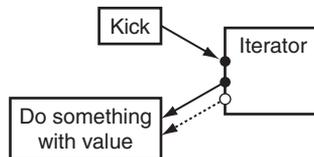
The boxes represent actions, as in a regular flow chart. When an iterator is kicked, it emits a value, which is represented by the dotted line coming out of the left-hand side. Solid arrows represent the flow of control, dotted arrows the flow of data.
