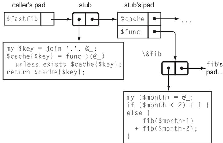
FIGURE 3.2 The data structure manufactured by `memoize`.
