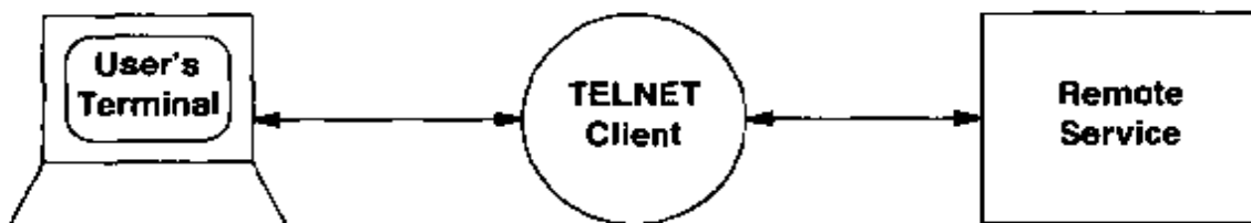
Figure 25.1 Conceptual role of a TELNET client. The client must transfer characters from the user's keyboard to a remote service, and it must transfer characters from the remote service to the user's display.
