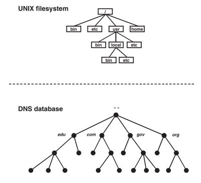
**FIGURE 16.1** The structure of the DNS space.
