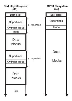
FIGURE 6.2 The filesystem layout.
