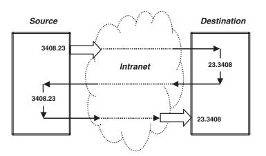
**FIGURE 15.3** Dynamically allocated port numbers.
