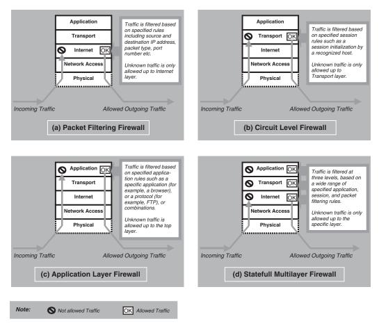
FIGURE 25.5 Basic firewall types.
