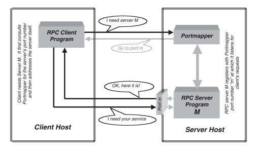
**FIGURE 15.5** The RPC client/server communication.
