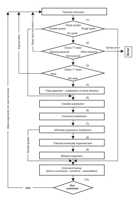
FIGURE 3.2 Shell processing of the command line.
