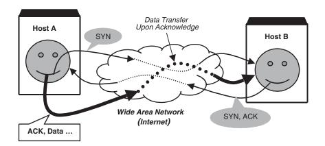
FIGURE 14.11 Three-way handshake.
