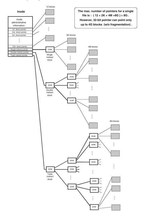
**FIGURE 6.4** File layout on a disk.
