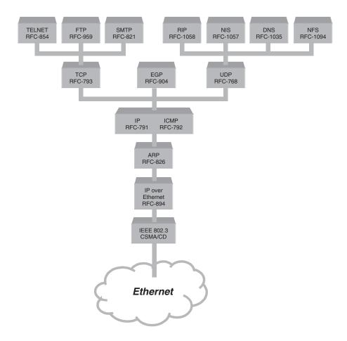
**FIGURE 14.12** The hierarchy of TCP/IP protocols.
