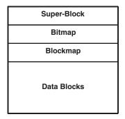
**FIGURE 6.8** The snapshot filesystem structure.
