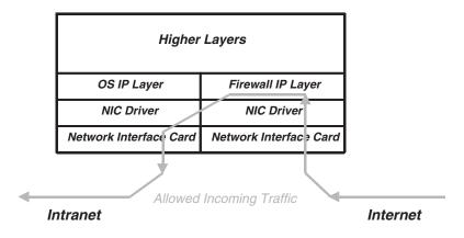
**FIGURE 25.4** Firewall IP layer.
