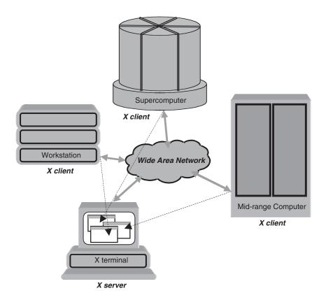
**FIGURE 22.1** An X server with multiple X clients.
