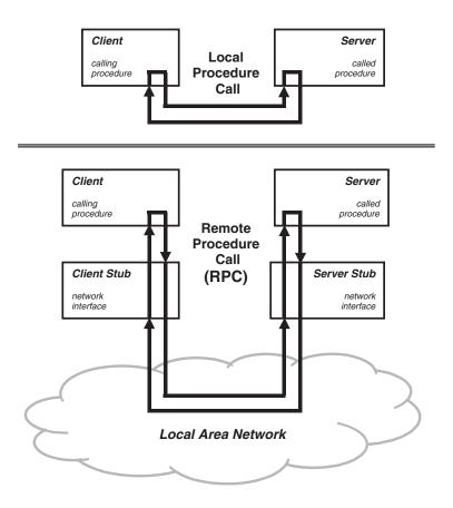
FIGURE 15.4 Local and remote procedure calling.
