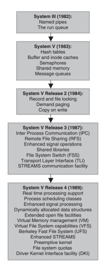
**FIGURE 1.2** The development of ATT UNIX.
