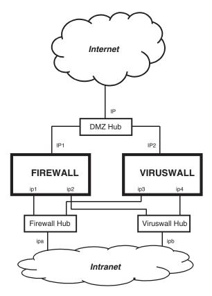
**FIGURE 25.6** Firewall-viruswall configuration.
