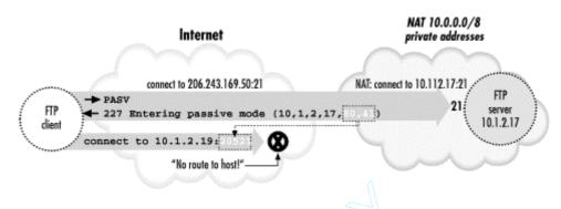
Figure 11.6. Server-side NAT prevents passive-mode FTP transfers
