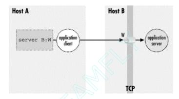
Figure 9.3. Direct client/server connection (no forwarding)
