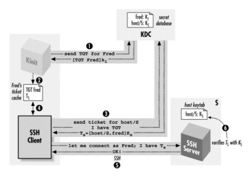
Figure 11.12. SSH with Kerberos authentication
